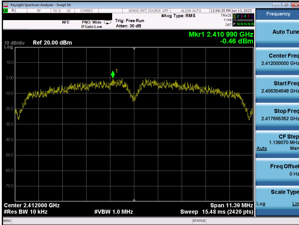
Plot 7-61. Power Spectral Density Plot MIMO ANT2 (802.11b – Ch. 1)
