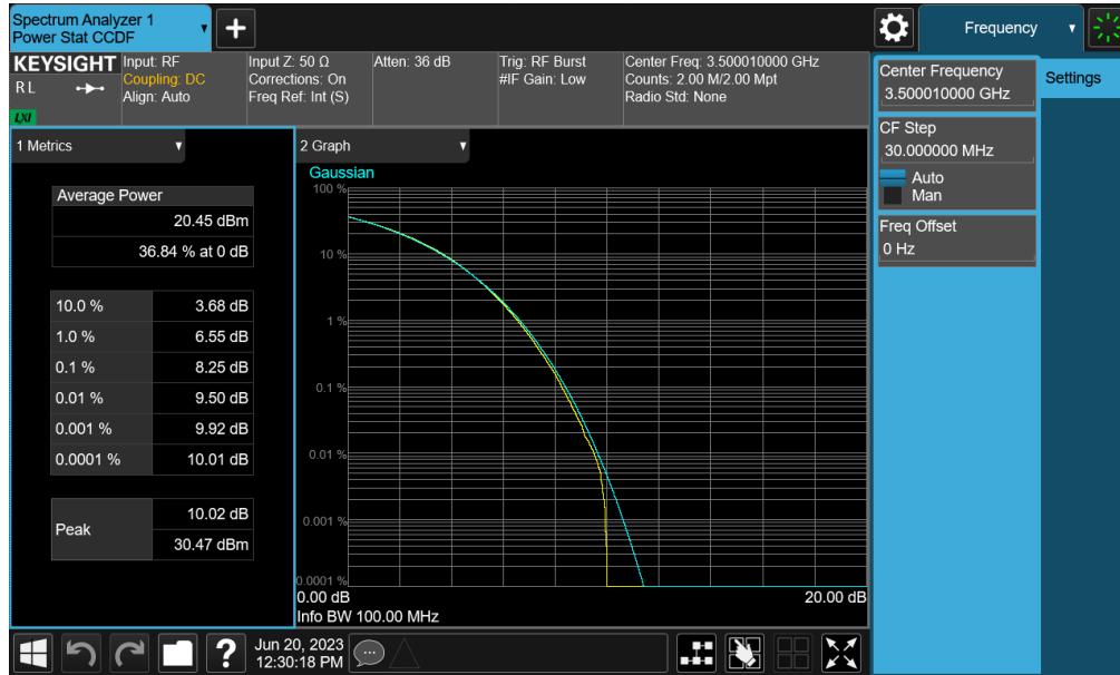
Plot 7-78. PAR Plot (NR Band n77 (DoD) - 100MHz CP-OFDM 256-QAM - Full RB - Ant F)
