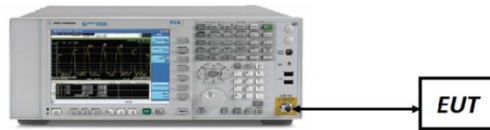
Figure 7-4. Test Instrument & Measurement Setup
