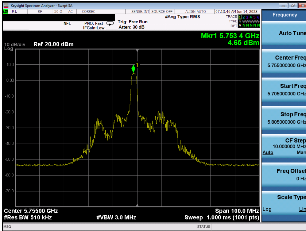
Plot 7-85. Power Spectral Density Plot MIMO ANT1 (40MHz BW 802.11ax – 26 Tones (UNII Band 3) – Ch. 151)
