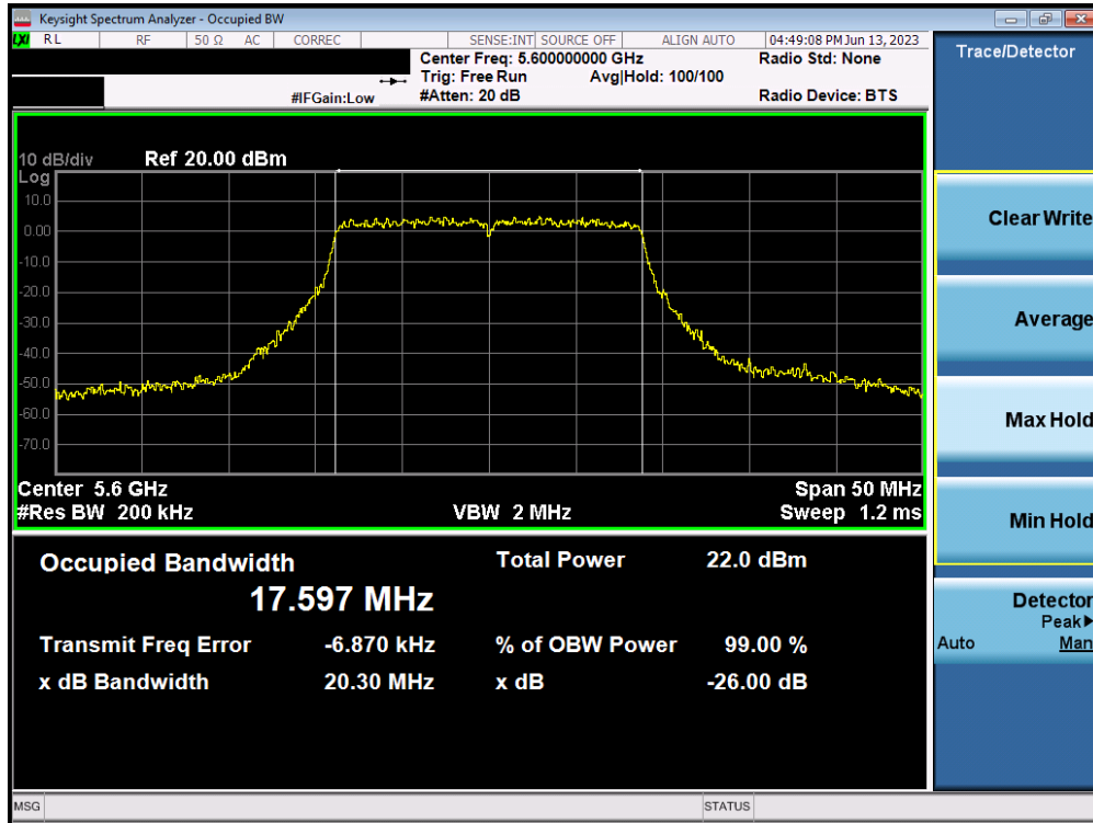
Plot 7-18. 26dB Bandwidth Plot MIMO ANT1 (20MHz BW 802.11n (UNII Band 2C) – Ch. 120)
