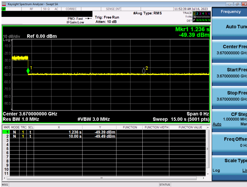
Plot 7-76. Run#2 End User Device Discontinues Operations within 10s
