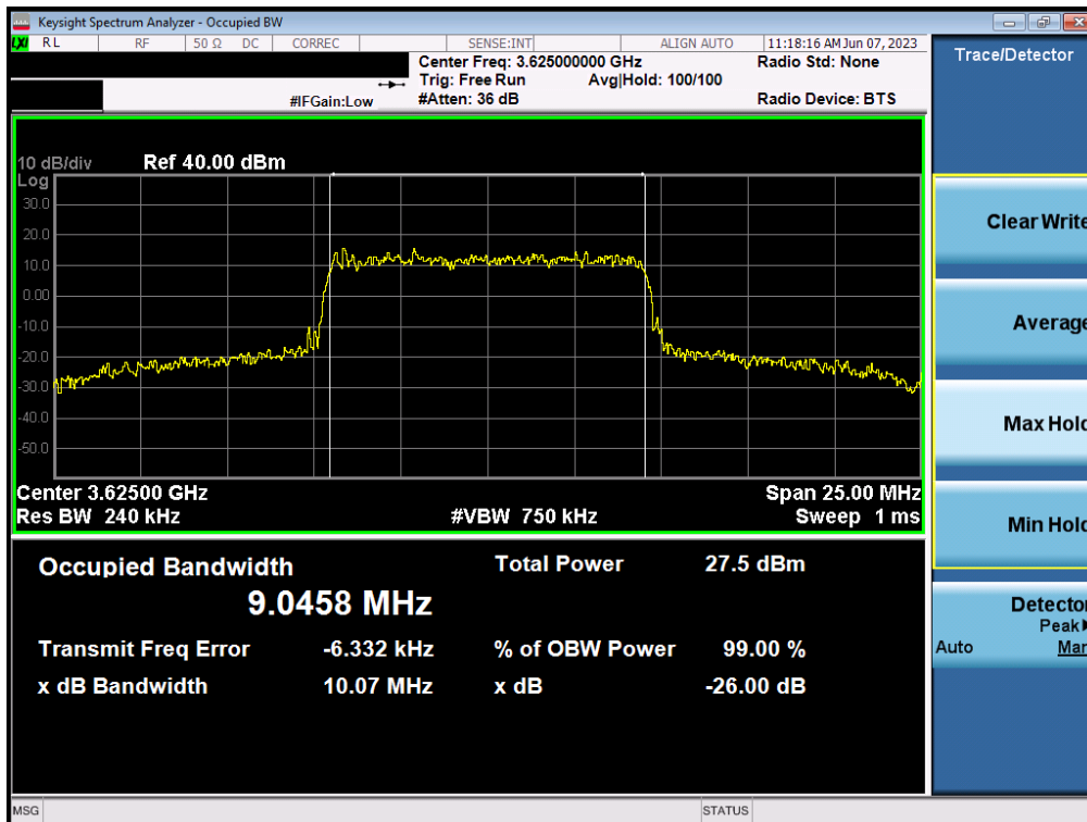
Plot 7-13. Occupied Bandwidth Plot (LTE Band 48 - 10MHz QPSK - Full RB Configuration - Ant1)
