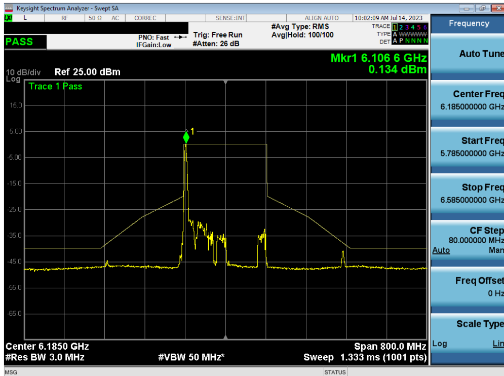
Plot 7-204. In-Band Emission Plot MIMO ANT2 (160MHz BW 802.11ax (26 Tones) (UNII Band 5) – Ch. 47) – LPI
