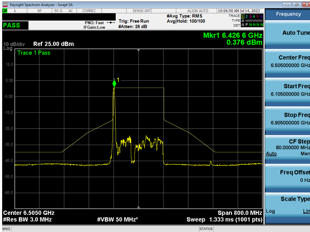
Plot 7-212. In-Band Emission Plot MIMO ANT2 (160MHz BW 802.11ax (26 Tones) (UNII Band 6) – Ch. 111)
