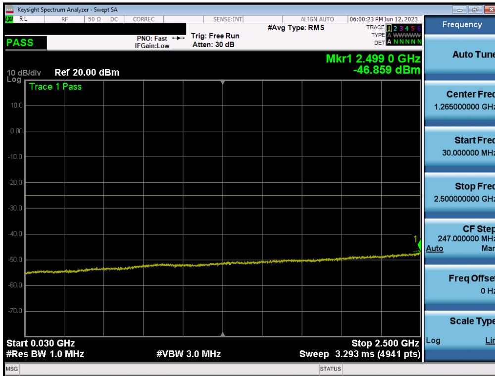
Plot 7-144. Conducted Spurious Plot (LTE Band 7 - 20MHz QPSK - RB Size 1, RB Offset 0 - Mid Channel - Ant2)
