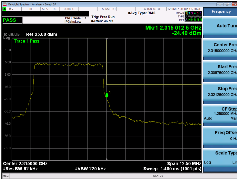
Plot 7-191. Upper Band Edge Plot (NR Band n30 - 5MHz CP-OFDM-QPSK – Full RB - Ant1)
