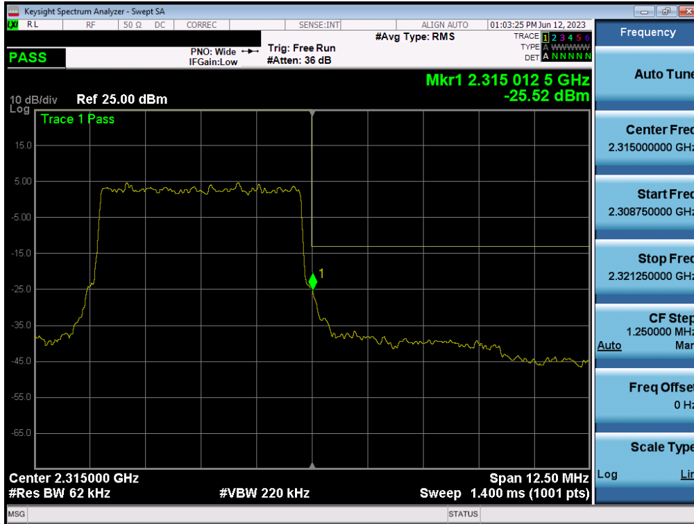
Plot 7-215. Upper Band Edge Plot (NR Band n30 - 5MHz CP-OFDM-QPSK – Full RB - Ant2)
