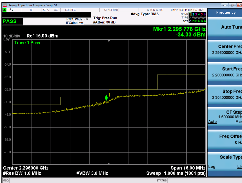
Plot 7-167. Extended Lower Band Edge Plot (LTE Band 30 - 10MHz QPSK – Full RB - Ant1)
