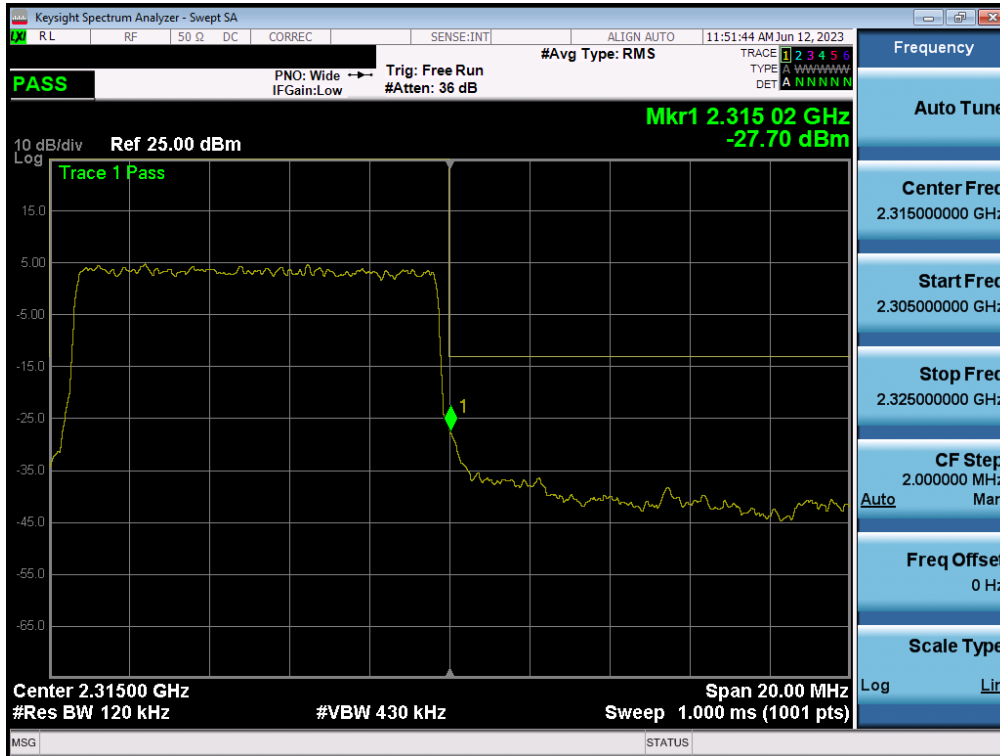
Plot 7-187. Upper Band Edge Plot (NR Band n30 - 10MHz CP-OFDM-QPSK – Full RB - Ant1)
