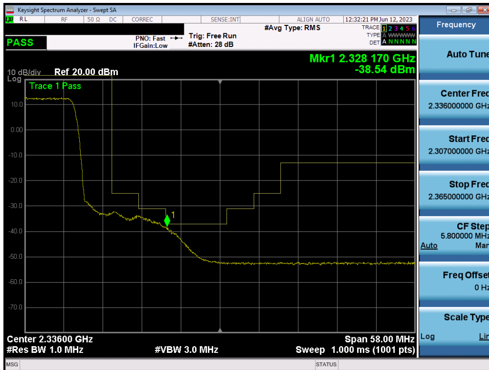
Plot 7-188. Extended Upper Band Edge Plot (NR Band n30 - 10MHz CP-OFDM-QPSK – Full RB - Ant1)
