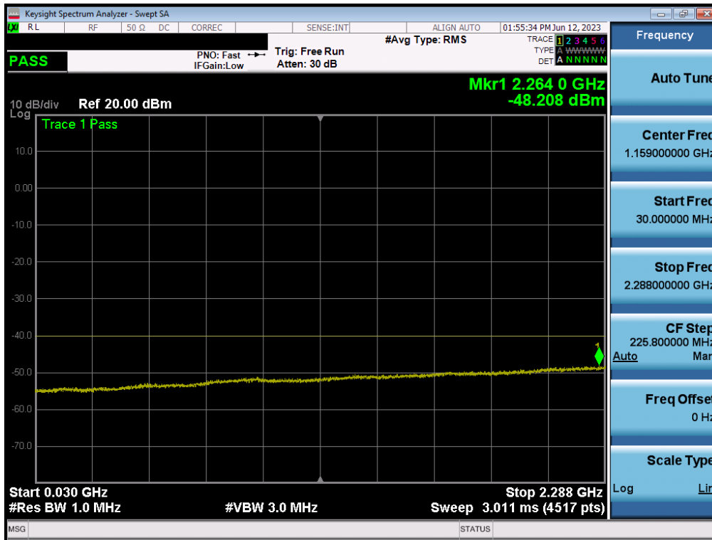
Plot 7-141. Conducted Spurious Plot (LTE Band 30 - 10MHz QPSK - RB Size 1, RB Offset 0 - Ant2)
