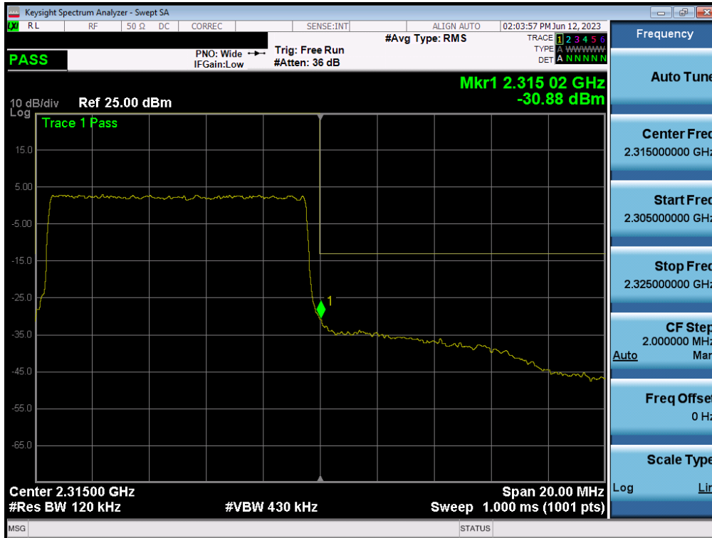
Plot 7-198. Upper Band Edge Plot (LTE Band 30 - 10MHz QPSK – Full RB - Ant2)
