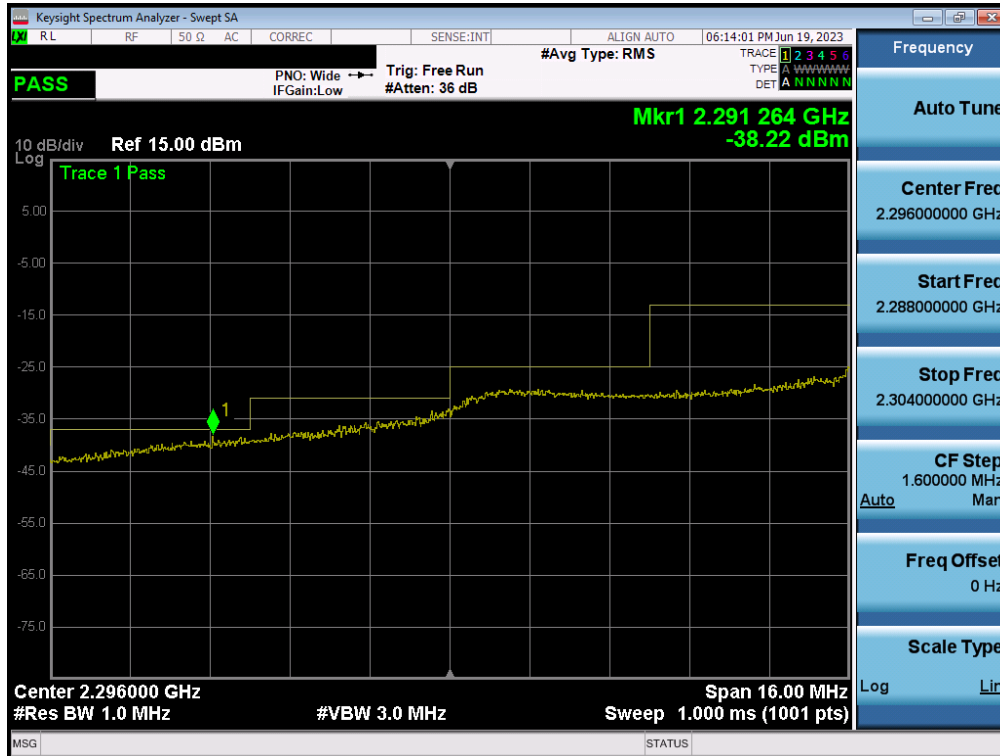
Plot 7-197. Extended Lower Band Edge Plot (LTE Band 30 - 10MHz QPSK – Full RB - Ant2)
