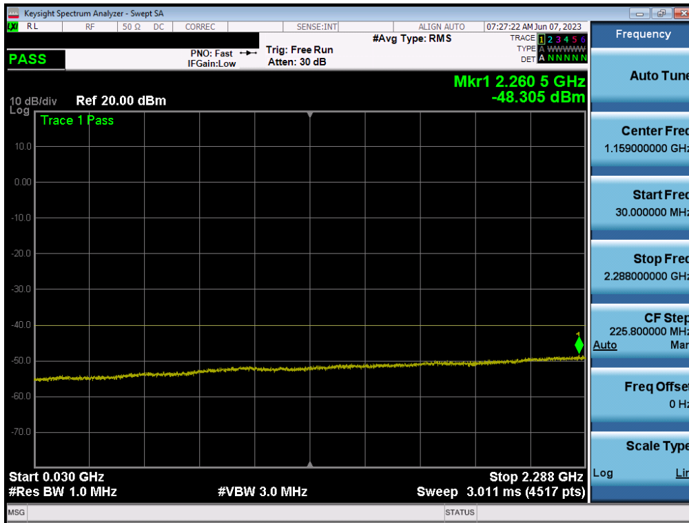
Plot 7-113. Conducted Spurious Plot (LTE Band 30 - 10MHz QPSK - RB Size 1, RB Offset 0 - Ant1)
