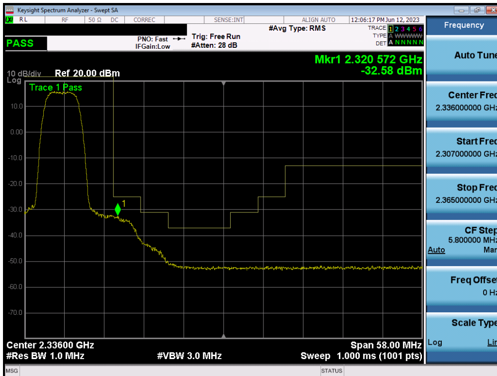
Plot 7-192. Extended Upper Band Edge Plot (NR Band n30 - 5MHz CP-OFDM-QPSK – Full RB - Ant1)
