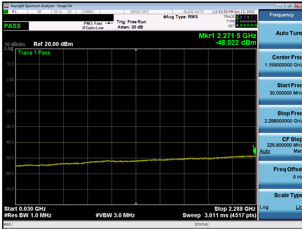
Plot 7-162. Conducted Spurious Plot (NR Band n30 - 10MHz QPSK - RB Size 1, RB Offset 0 – Ant2)
