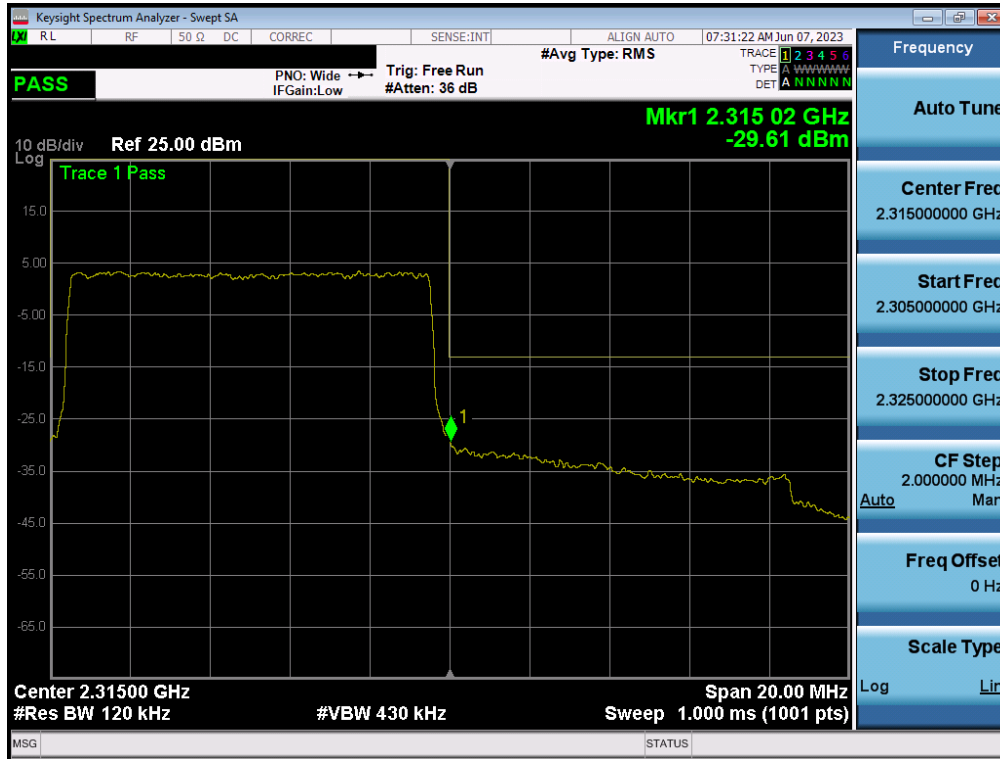
Plot 7-168. Upper Band Edge Plot (LTE Band 30 - 10MHz QPSK – Full RB - Ant1)
