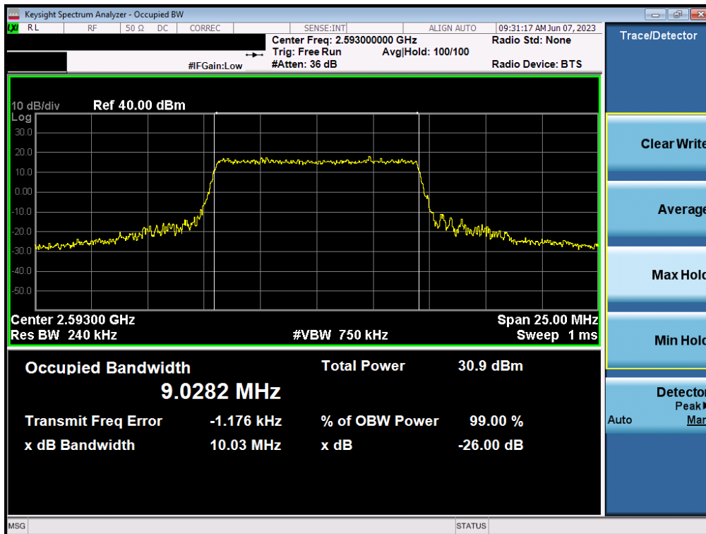
Plot 7-39. Occupied Bandwidth Plot (LTE Band 41(PC3)/38 - 10MHz 16-QAM - Full RB - Ant1)
