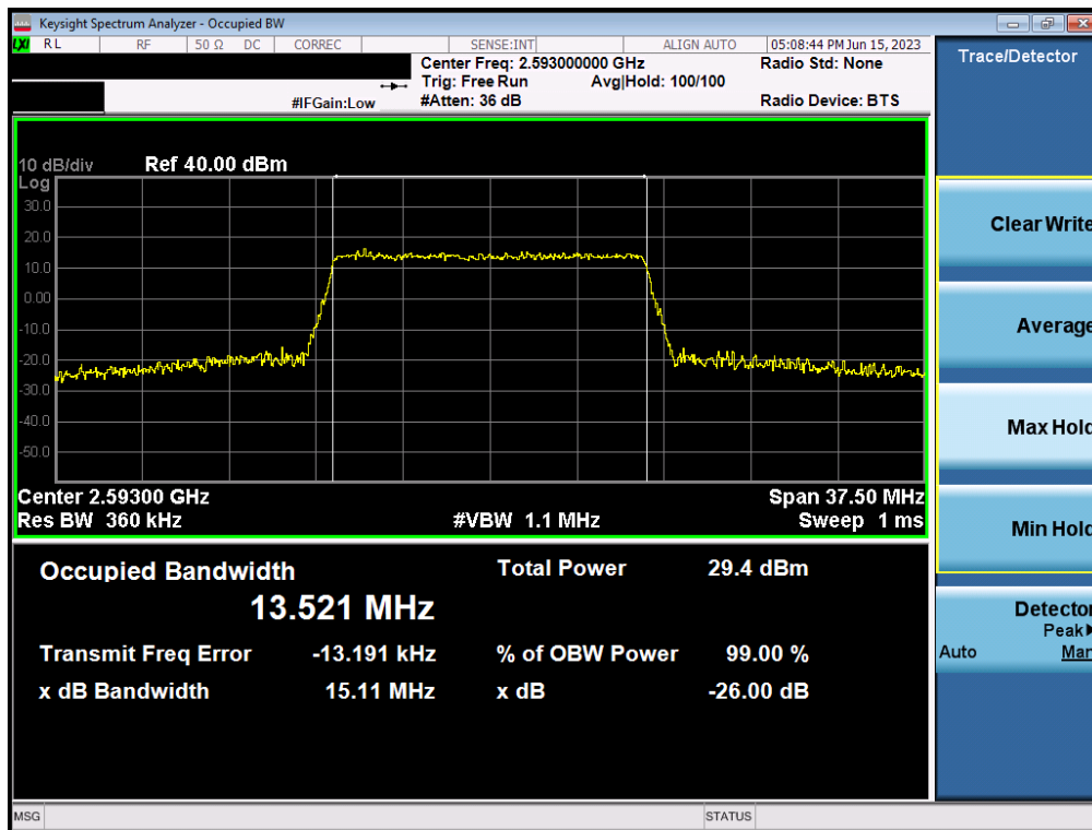
Plot 7-92. Occupied Bandwidth Plot (LTE Band 41(PC2) - 15MHz 16-QAM - Full RB - Ant2)
