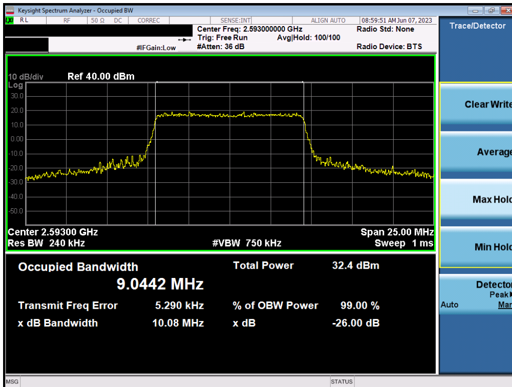
Plot 7-31. Occupied Bandwidth Plot (LTE Band 41(PCI) - 10MHz 16-QAM - Full RB - Ant1)
