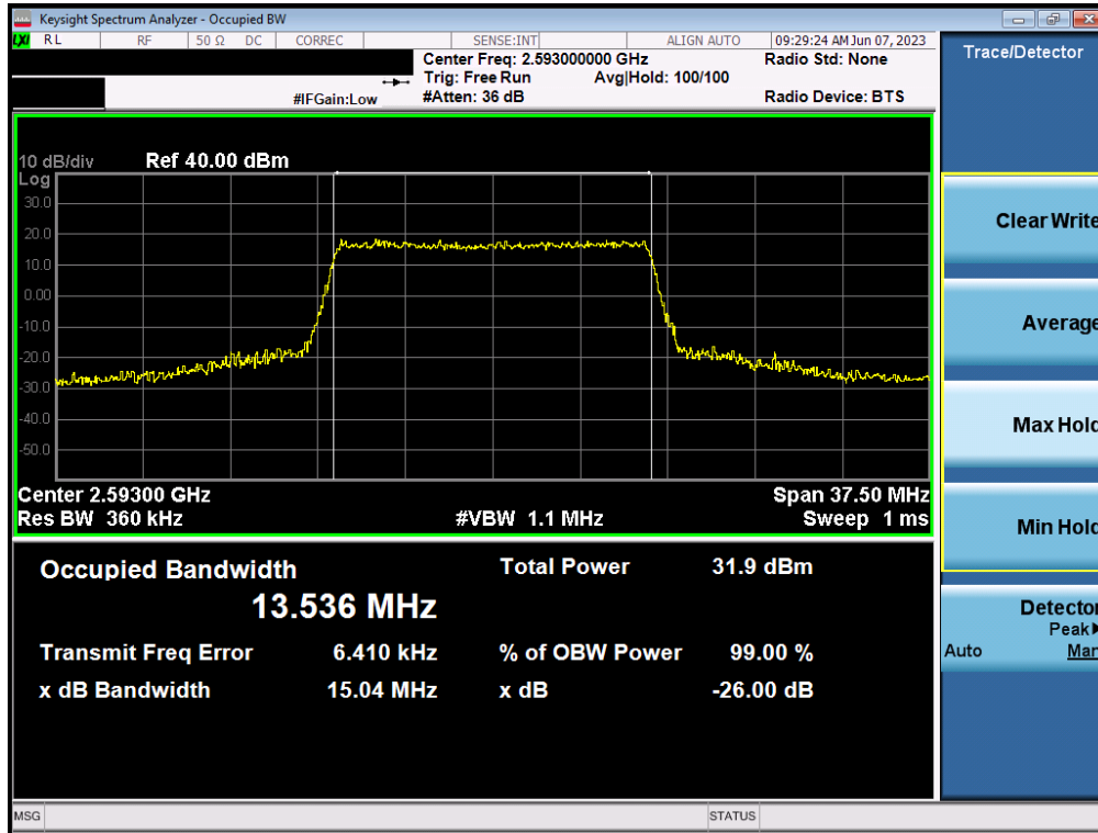
Plot 7-36. Occupied Bandwidth Plot (LTE Band 41(PC3)/38 - 15MHz QPSK - Full RB - Ant1)
