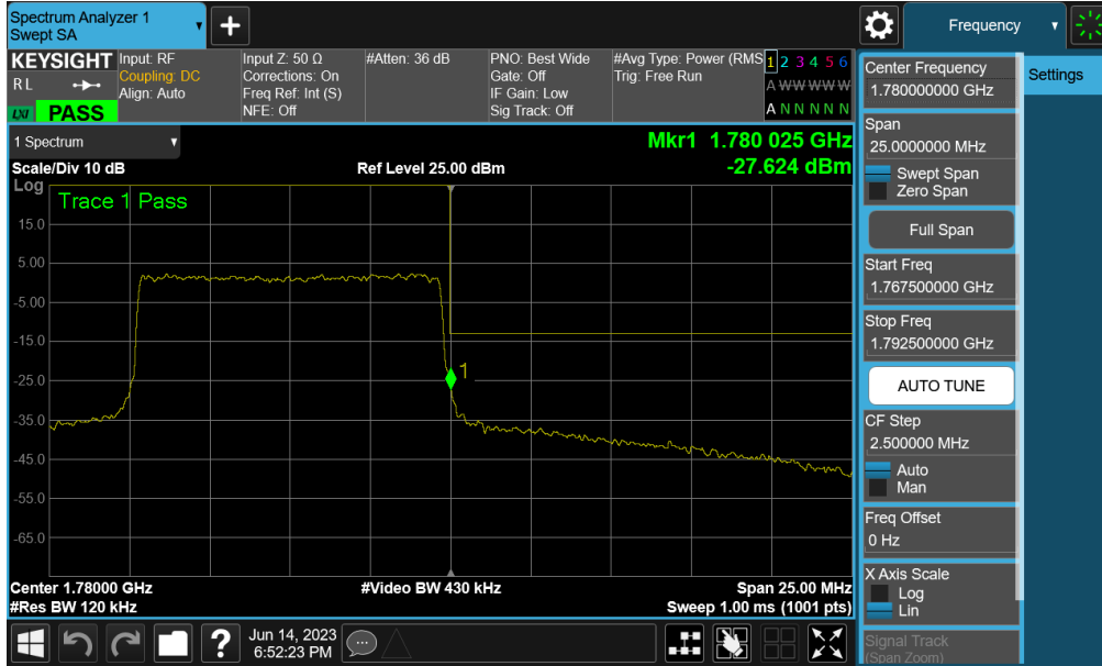
Plot 7-185. Upper Band Edge Plot (NR Band n66 – 10.0MHz - Full RB - ANT F)
