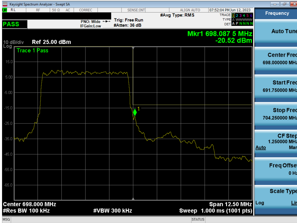
Plot 7-156. Upper Band Edge Plot (NR Band n71 – 5.0MHz - Full RB - ANT A)
