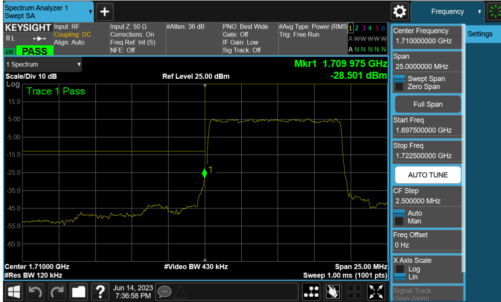
Plot 7-169. Lower Band Edge Plot (NR Band n66 – 10.0MHz - Full RB - ANT A)
