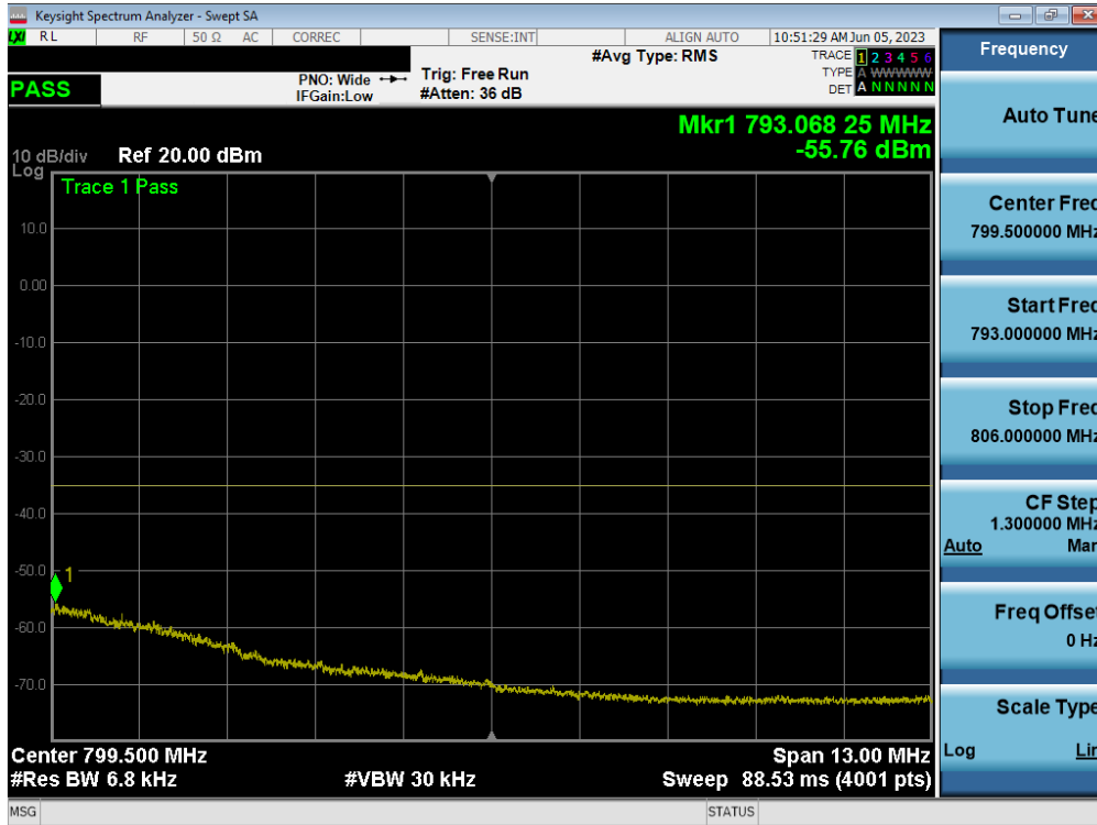
Plot 7-154. Upper Emission Mask Plot (LTE Band 13 - 5MHz QPSK – Full RB - ANT A)
