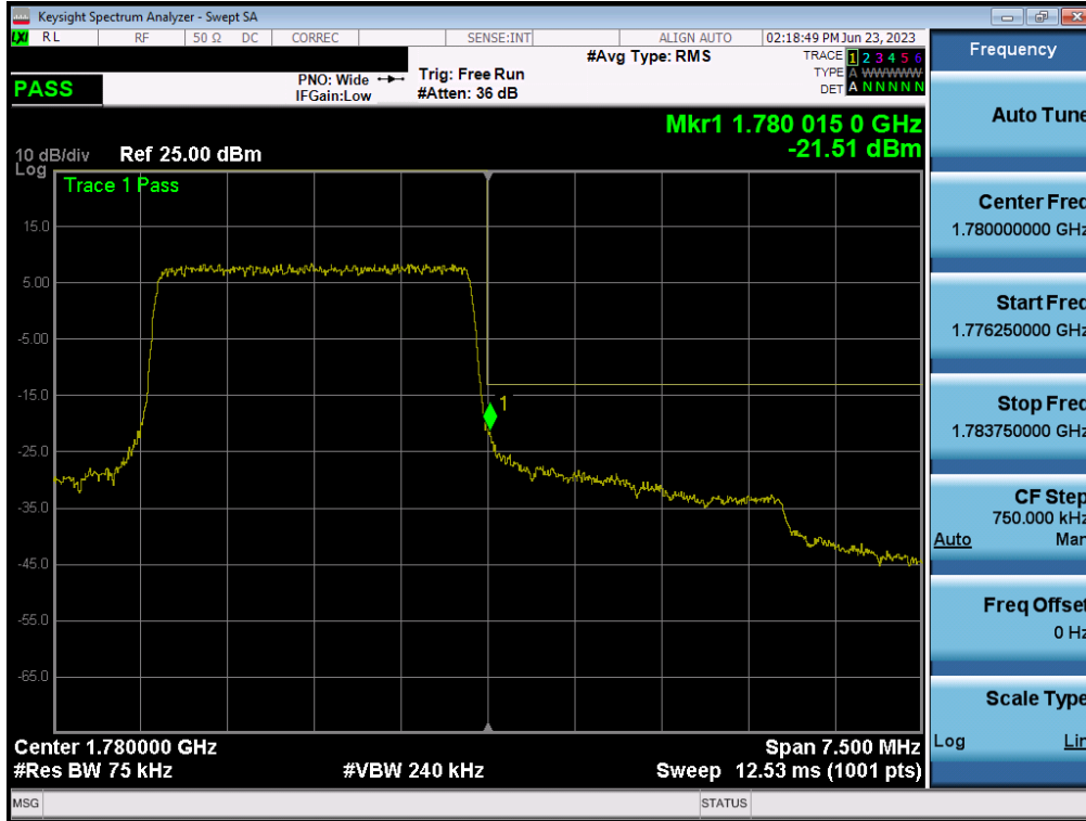
Plot 7-167. Upper Band Edge Plot (LTE Band 66 - 3MHz QPSK – Full RB - ANT A)
