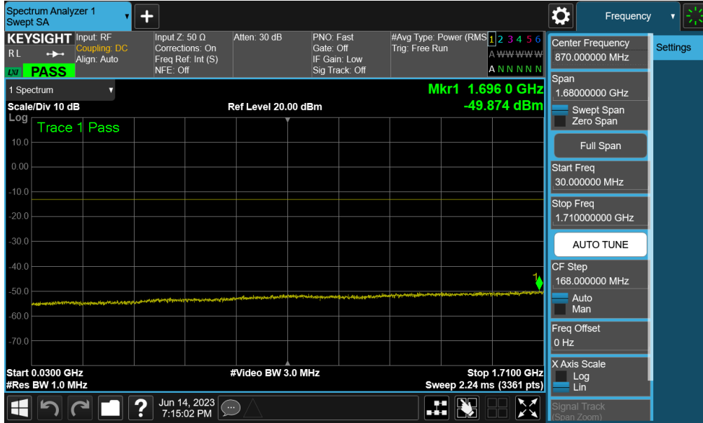
Plot 7-130. Conducted Spurious Plot (NR Band n66 - 40.0MHz - 1 RB - High Channel - ANT A)
