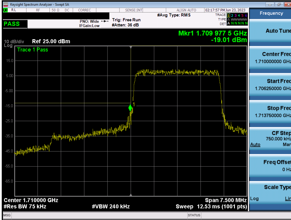
Plot 7-163. Lower Band Edge Plot (LTE Band 66/4 - 3MHz QPSK – Full RB - ANT A)
