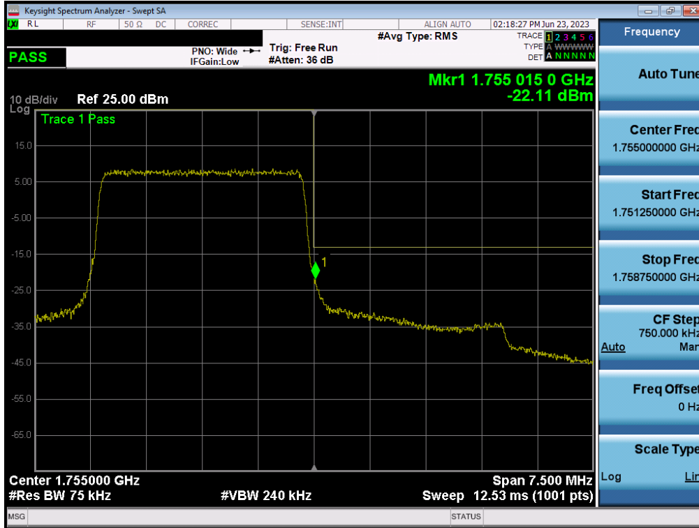
Plot 7-165. Upper Band Edge Plot (LTE Band 4 - 3MHz QPSK – Full RB - ANT A)
