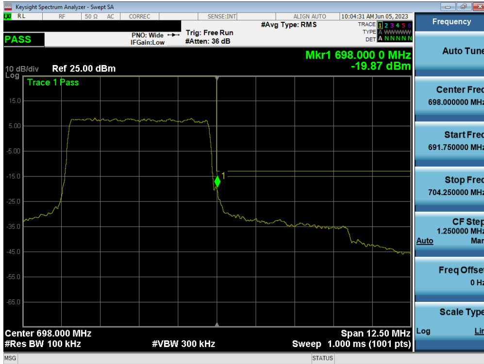
Plot 7-148. Upper Band Edge Plot (LTE Band 71 - 5MHz QPSK – Full RB - ANT A)
