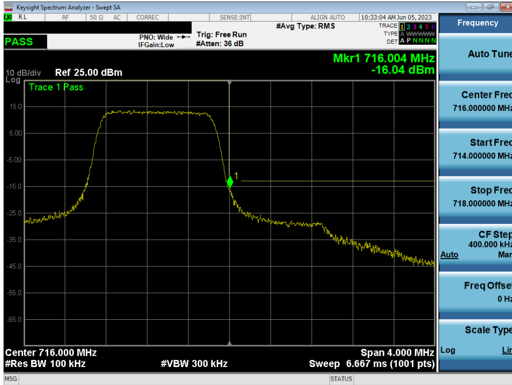
Plot 7-150. Upper Band Edge Plot (LTE Band 12 – 1.4MHz QPSK – Full RB - ANT A)
