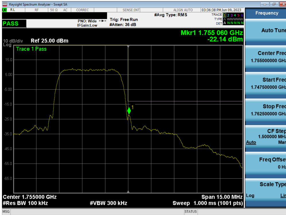
Plot 7-161. Upper Band Edge Plot (WCDMA AWS – Ch. 1513 – ANT A)
