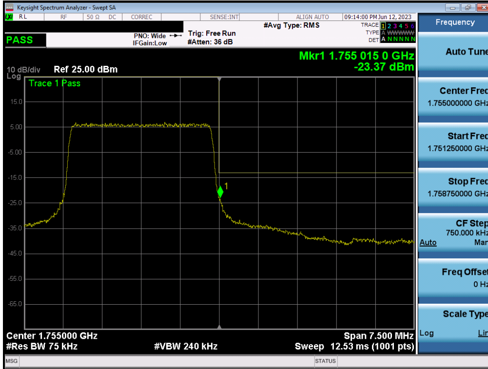
Plot 7-179. Upper Band Edge Plot (LTE Band 4 - 3MHz QPSK – Full RB - ANT F)
