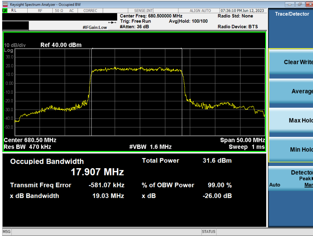
Plot 7-21. Occupied Bandwidth Plot (NR Band n71 - 20MHz DFT-s-OFDM BPSK - Full RB – ANT A)
