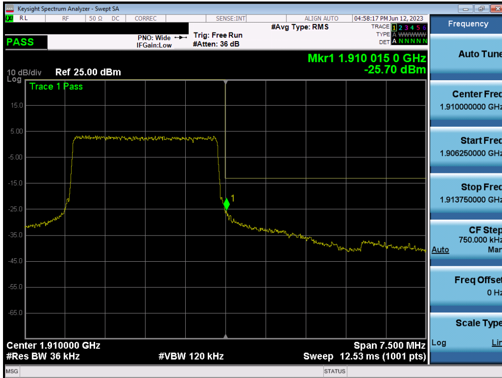
Plot 7-110. Upper Band Edge Plot (LTE Band 2 – 3MHz QPSK – Full RB - Ant F)
