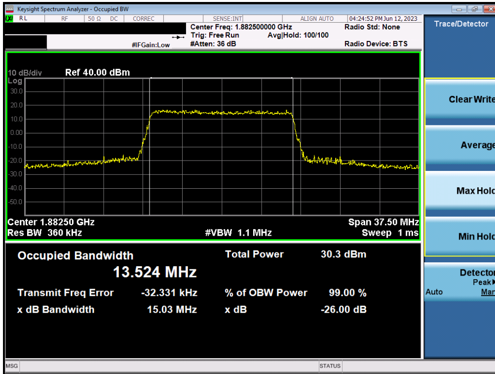
Plot 7-39. Occupied Bandwidth Plot (LTE Band 25/2 - 15MHz QPSK - Full RB - Ant F)
