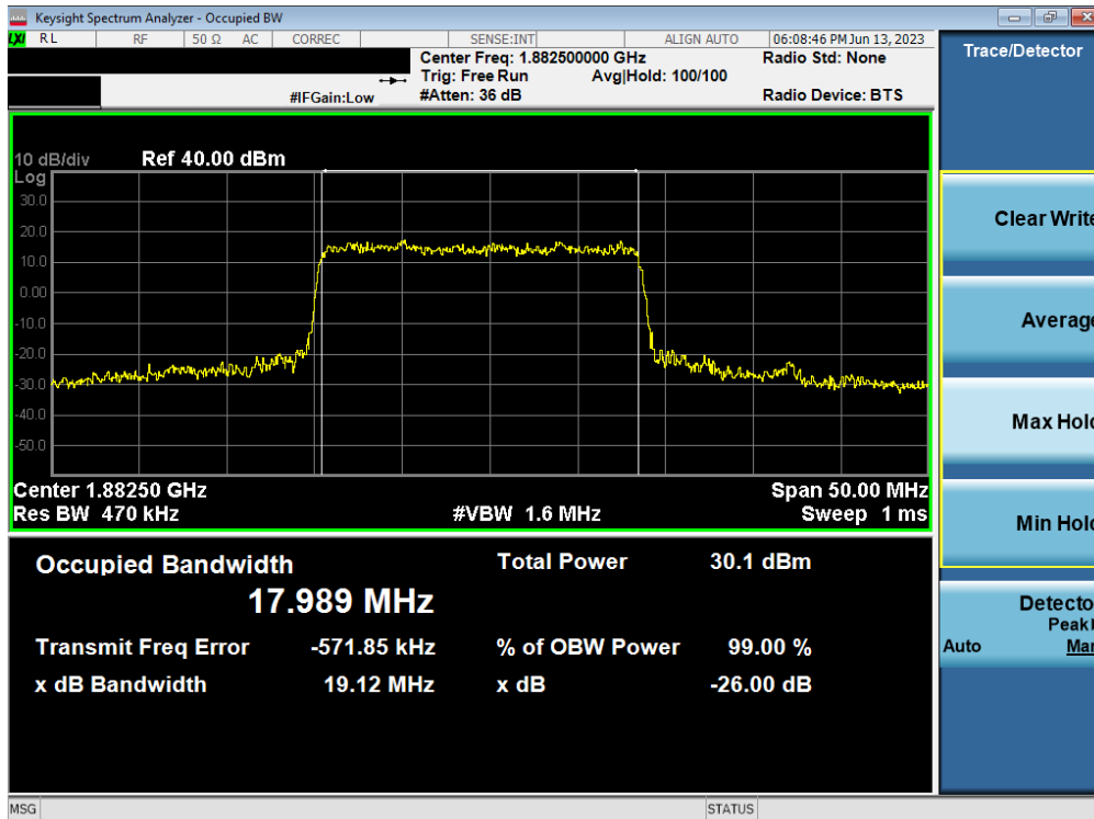
Plot 7-58. Occupied Bandwidth Plot (NR Band n25/2 - 20.0MHz DFT-s-OFDM BPSK - Full RB - ANT F)
