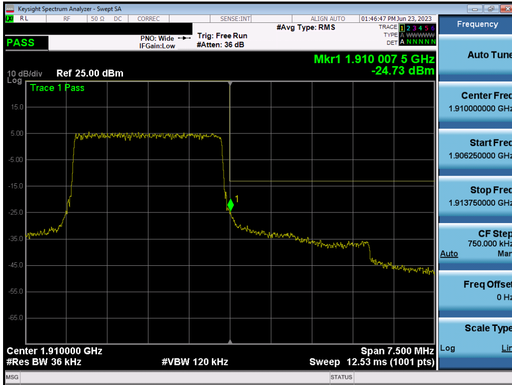
Plot 7-98. Upper Band Edge Plot (LTE Band 2 - 3MHz QPSK – Full RB - Ant A)
