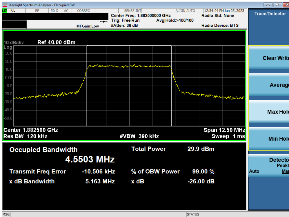
Plot 7-11. Occupied Bandwidth Plot (LTE Band 25/2 - 5MHz 16-QAM - Full RB - Ant A)
