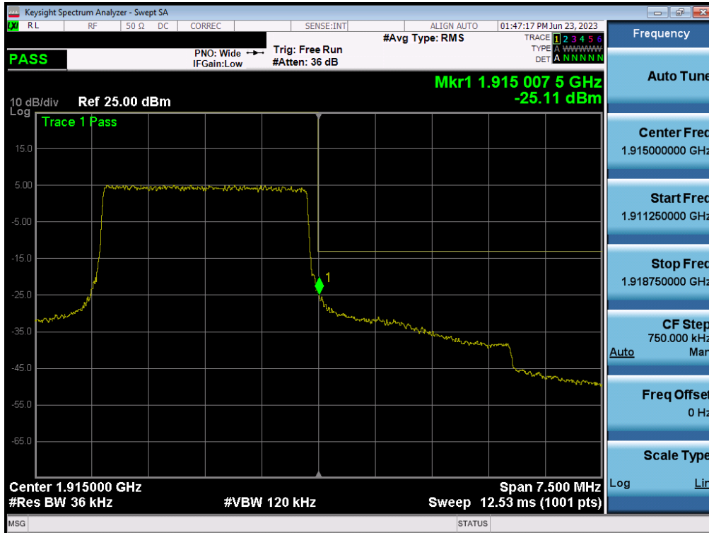
Plot 7-100. Upper Band Edge Plot (LTE Band 25 - 3MHz QPSK – Full RB - Ant A)
