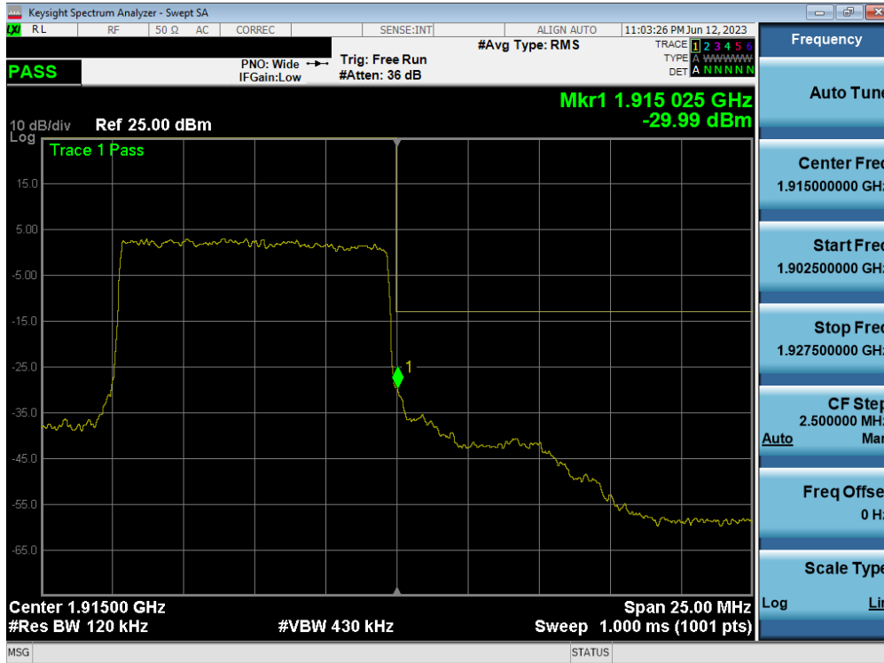
Plot 7-106. Upper Band Edge Plot (NR Band n25 - 10MHz QPSK – Full RB - Ant A)
