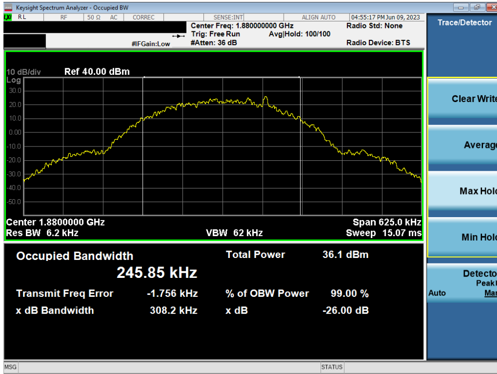
Plot 7-1. Occupied Bandwidth Plot (GPRS, Ch. 661 - Ant A)
