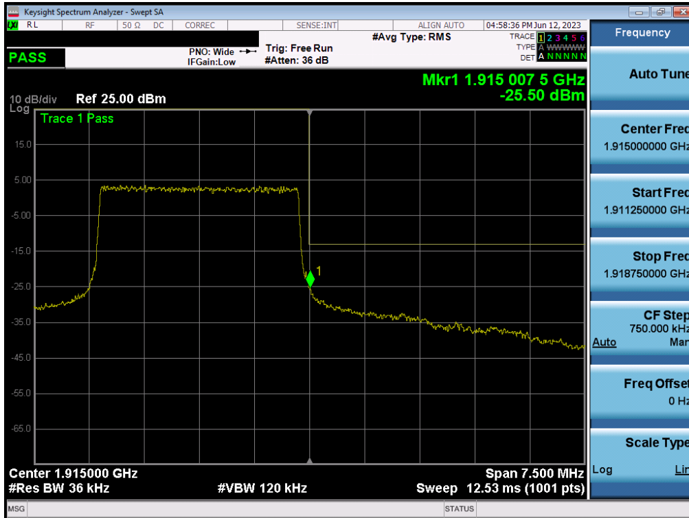
Plot 7-112. Upper Band Edge Plot (LTE Band 25 – 3MHz QPSK – Full RB - Ant F)
