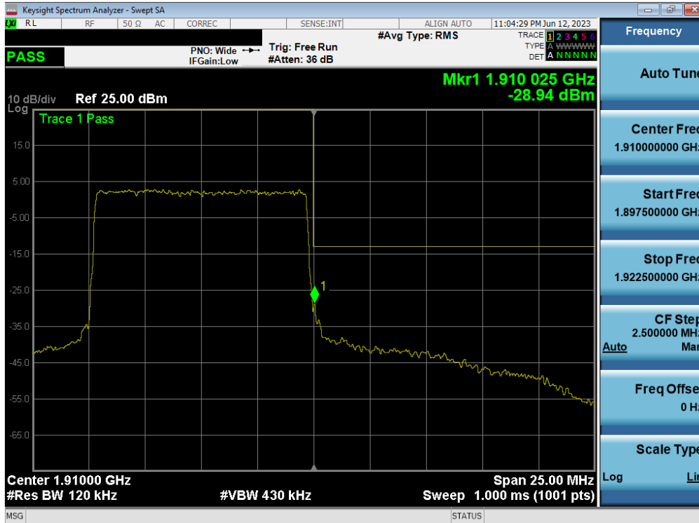
Plot 7-104. Upper Band Edge Plot (NR Band n2 - 10MHz QPSK – Full RB - Ant A)
