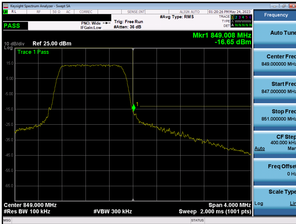
Plot 7-36. Upper Band Edge Plot (LTE Band 26/5 – 1.4MHz QPSK – Full RB Configuration)
