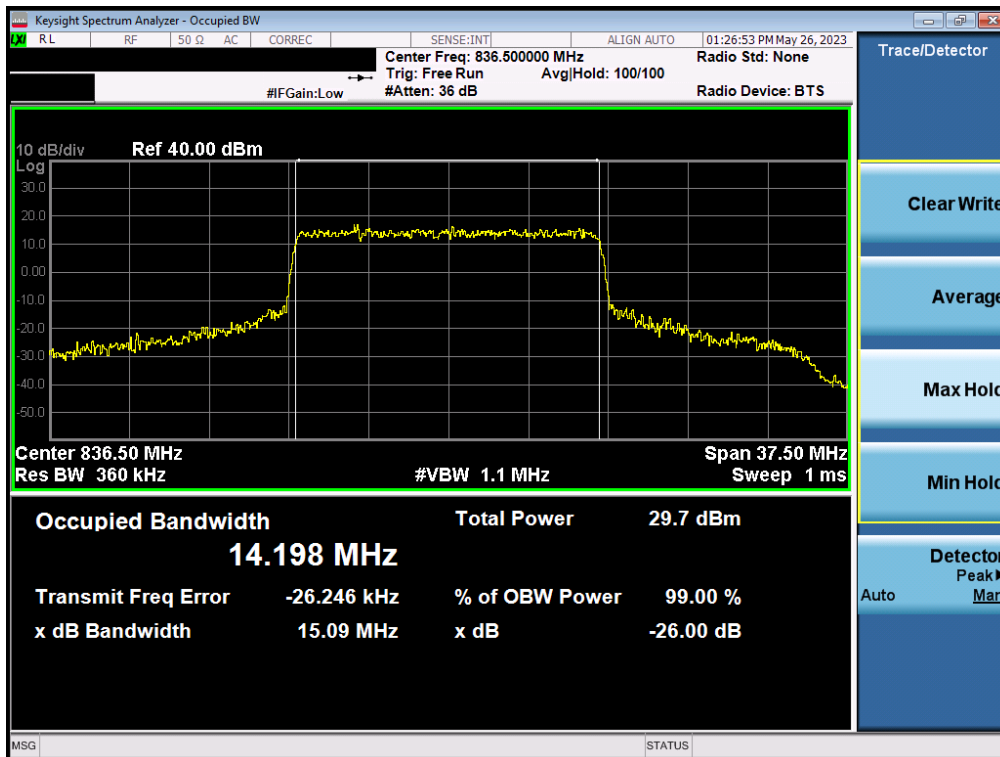
Plot 7-16. Occupied Bandwidth Plot (NR Band n26/5 - 15MHz 16-QAM - Full RB Configuration)
