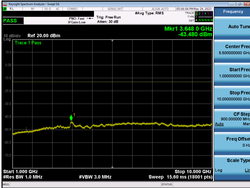
Plot 7-32. Conducted Spurious Plot (LTE Band 26 - 15MHz QPSK - RB Size 1, RB Offset 0)
