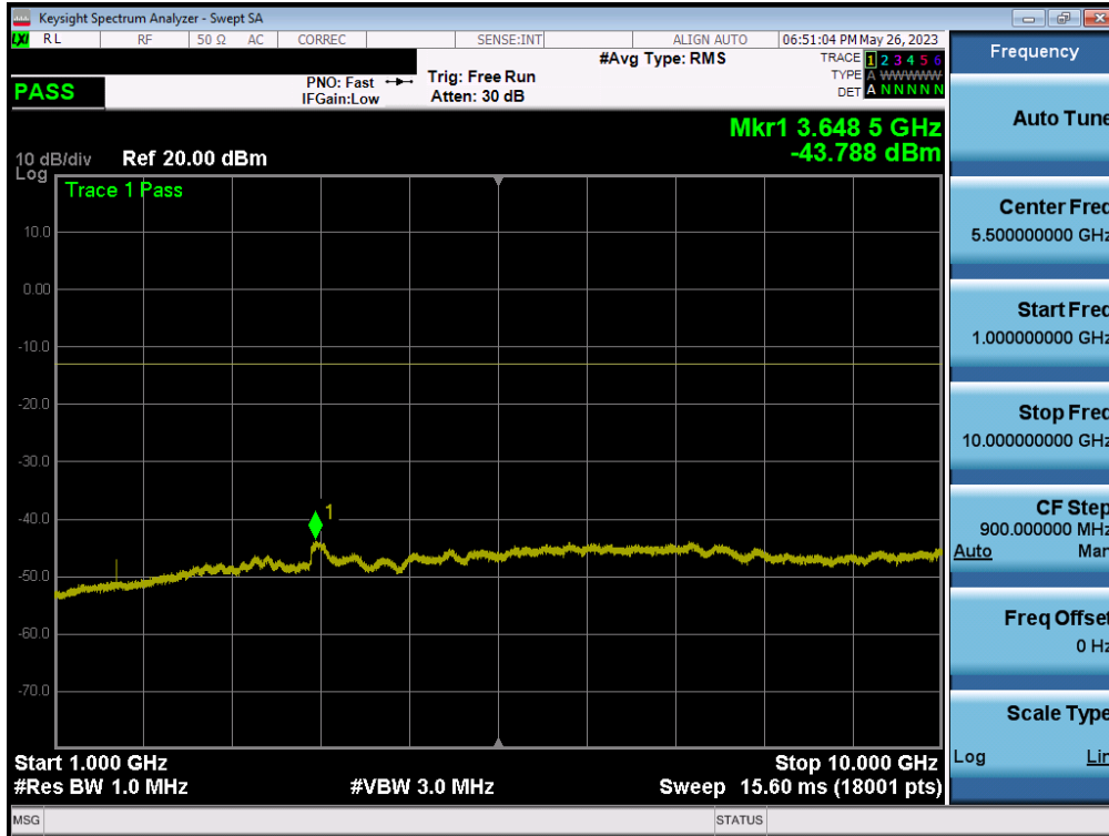
Plot 7-35. Conducted Spurious Plot (NR Band n26 - 20MHz QPSK - RB Size 1, RB Offset 0)
