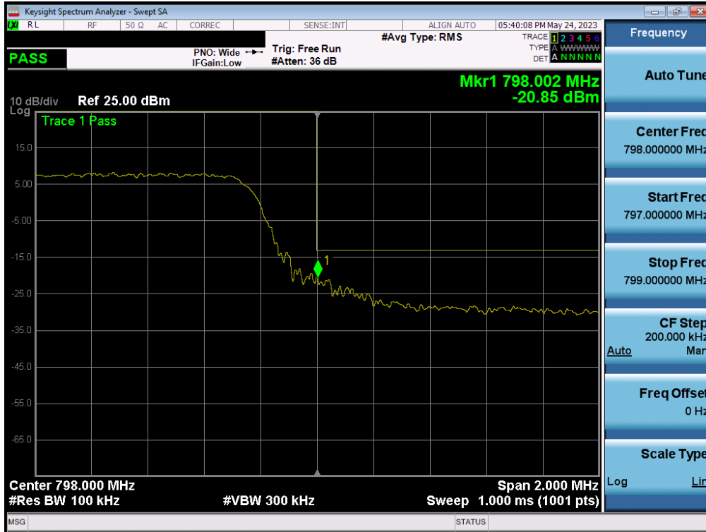
Plot 7-38. Upper Band Edge Plot (LTE Band 14, 5MHz QPSK)
