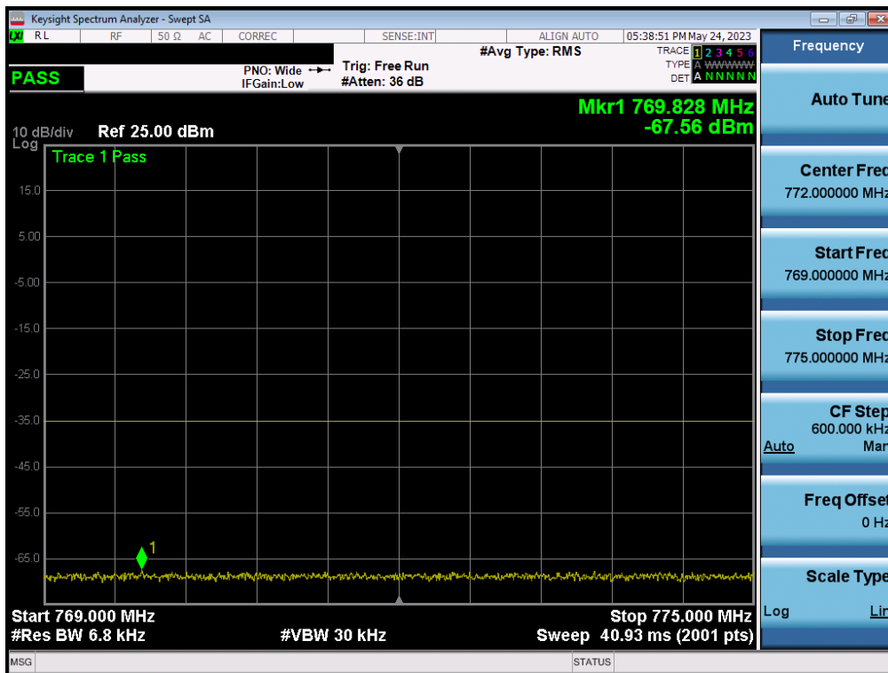
Plot 7-37. Lower Emission Mask Plot (LTE Band 14, 5MHz QPSK)
