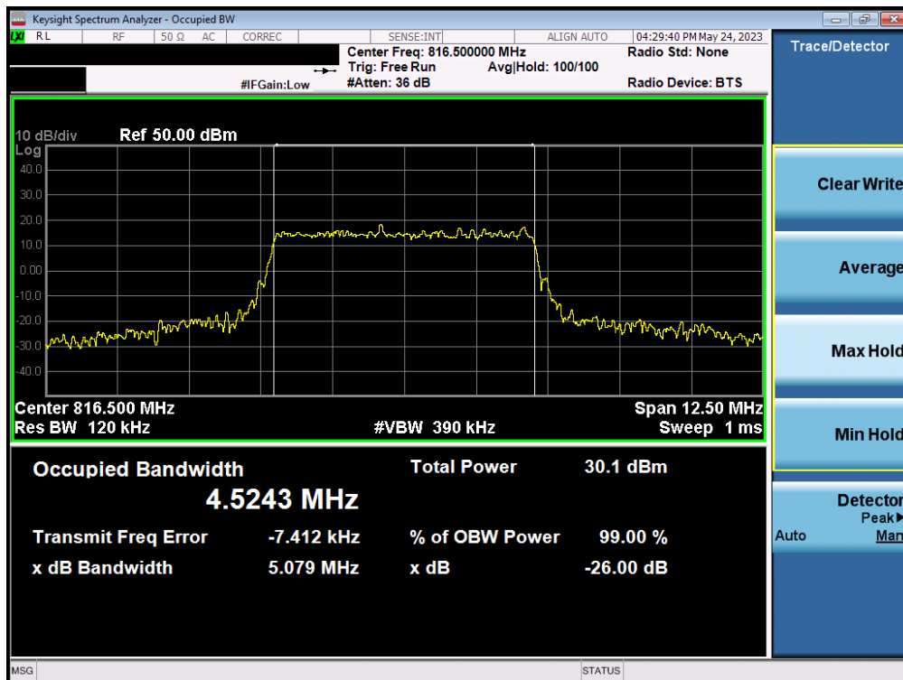
Plot 7-10. Occupied Bandwidth Plot (LTE Band 26 - 5MHz 16-QAM - Full RB Configuration)
