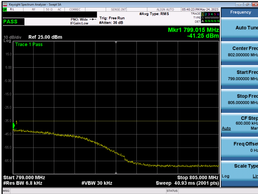
Plot 7-39. Upper Emission Mask Plot (LTE Band 14, 5MHz QPSK)
