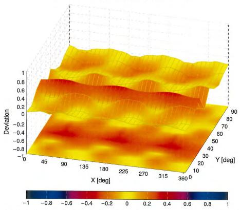
Probe isotropy for E<sub>tot</sub>: probe rotated  $\phi=0^\circ$  to 360°, tilted from field propagation direction  $\vec{k}$  Parallel to the field propagation ( $\psi=0^\circ-90^\circ$ ) at 30 GHz: deviation within  $\pm 0.28$  dB Parallel to the field propagation ( $\psi=0^\circ-90^\circ$ ) at 60 GHz: deviation within  $\pm 0.30$  dB
