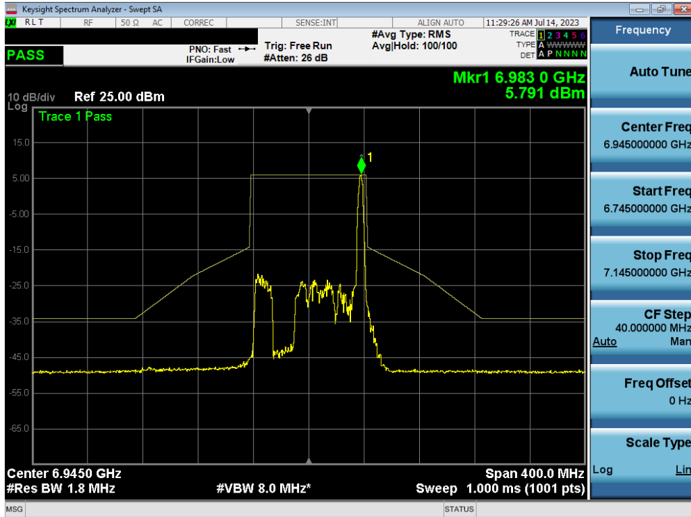
Plot 7-175. In-Band Emission Plot MIMO ANT2 (80MHz BW 802.11ax (26 Tones) (UNII Band 8) – Ch. 199)
