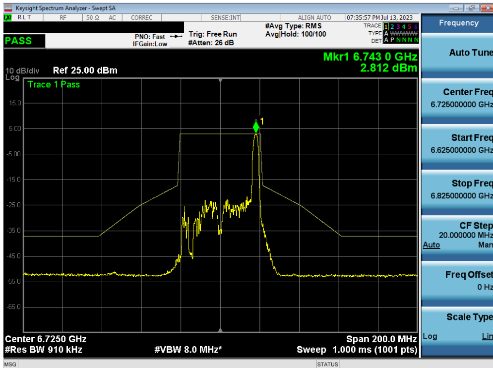
Plot 7-170. In-Band Emission Plot MIMO ANT2 (40MHz BW 802.11ax (26 Tones) (UNII Band 7) – Ch. 155)
