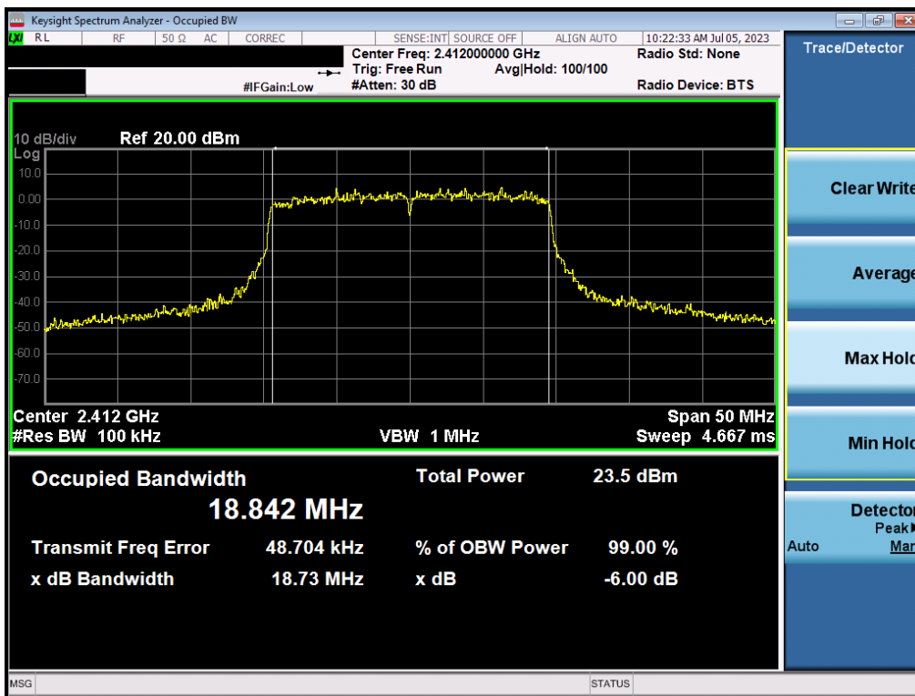
Plot 7-22. 6dB Bandwidth Plot MIMO ANT1 (802.1ax (2.4GHz) – Ch. 1)
