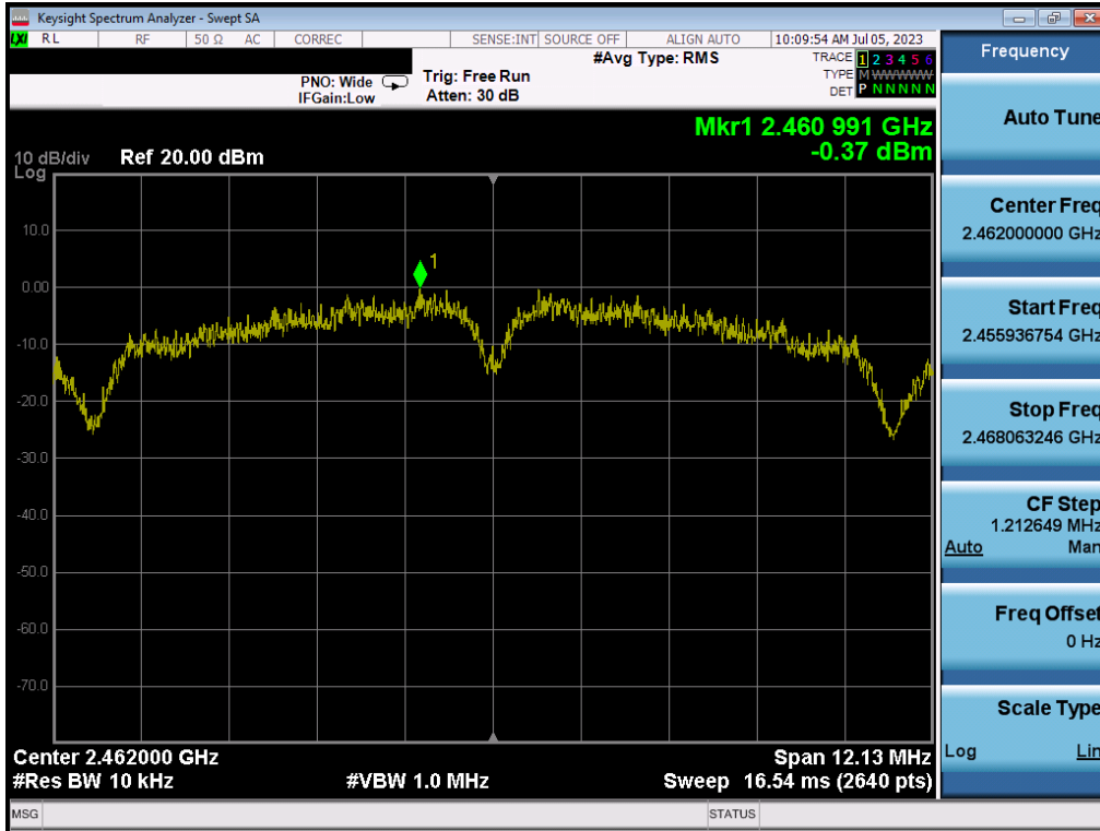
Plot 7-63. Power Spectral Density Plot MIMO ANT2 (802.11b – Ch. 11)
