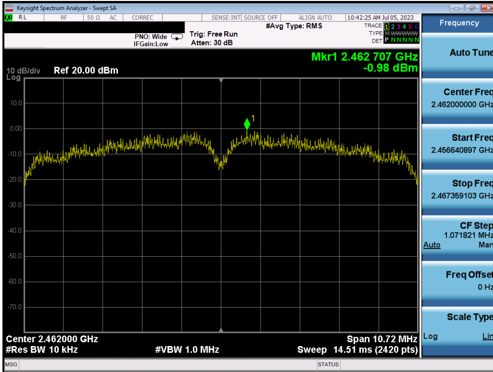
Plot 7-51. Power Spectral Density Plot MIMO ANT1 (802.11b – Ch. 11)
