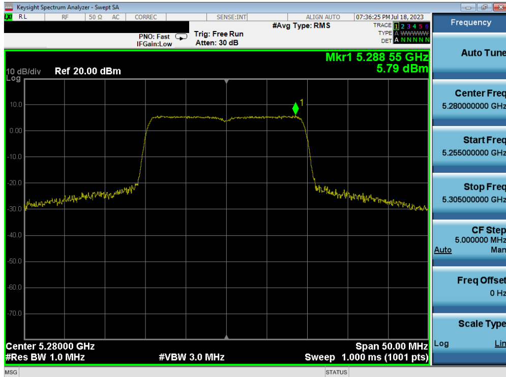
Plot 7-131. Power Spectral Density Plot MIMO ANT2 (20MHz BW 802.11ax – Full Tones (UNII Band 2A) – Ch. 56)
