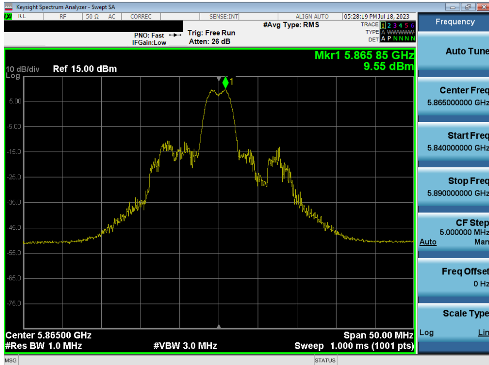
Plot 7-123. Power Spectral Density Plot MIMO ANT2 (20MHz BW 802.11ax – 26 Tones (UNII Band 4) – Ch. 173)
