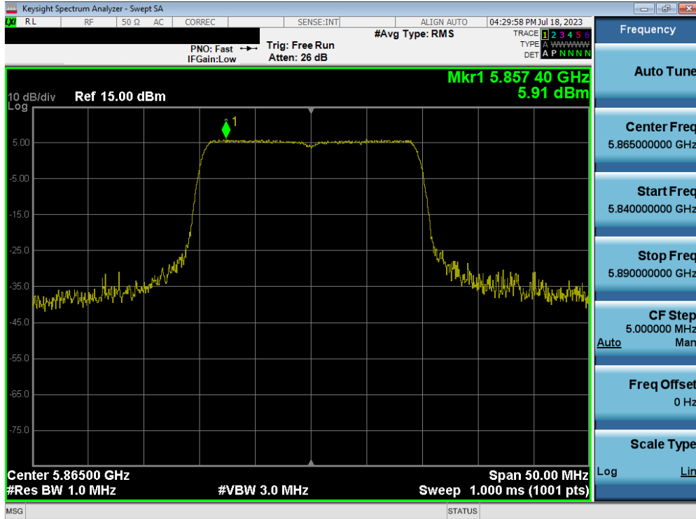
Plot 7-141. Power Spectral Density Plot MIMO ANT2 (20MHz BW 802.11ax – Full Tones (UNII Band 4) – Ch. 173)
