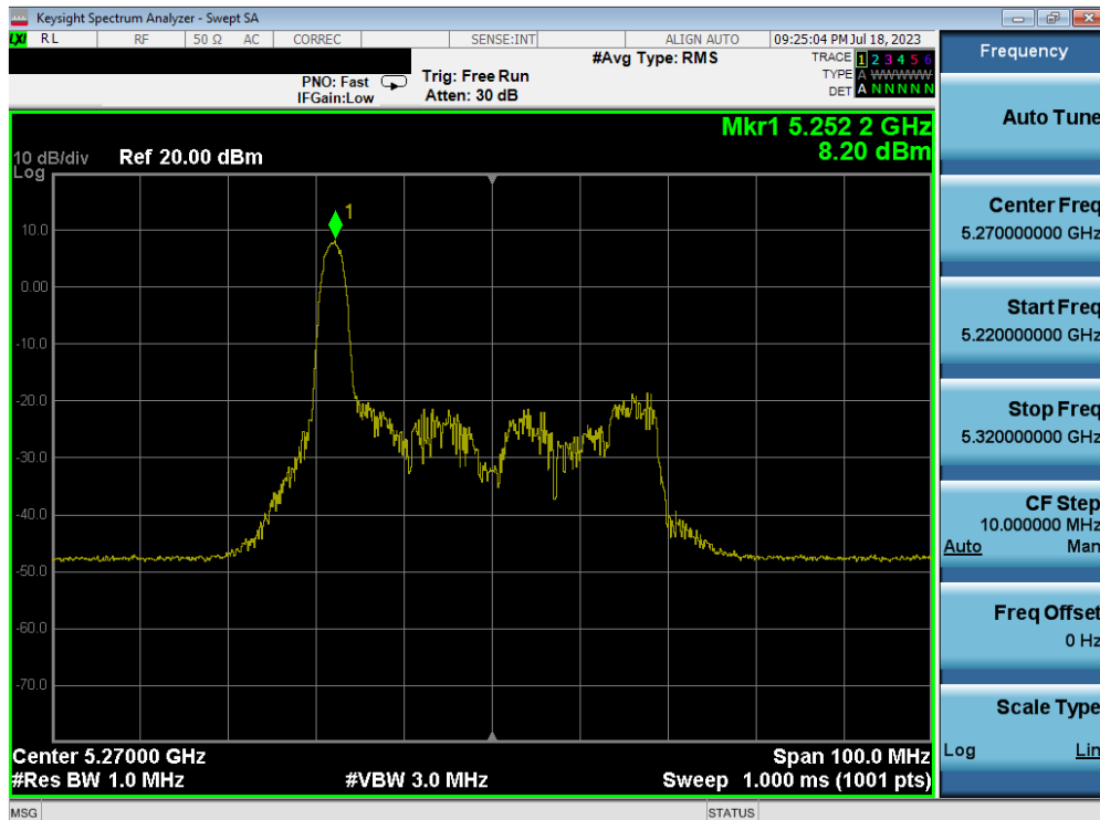
Plot 7-114. Power Spectral Density Plot MIMO ANT2 (40MHz BW 802.11ax – 26 Tones (UNII Band 2A) – Ch. 54)
