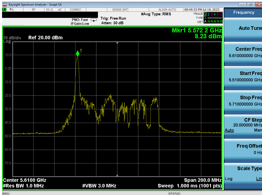
Plot 7-118. Power Spectral Density Plot MIMO ANT2 (80MHz BW 802.11ax – 26 Tones (UNII Band 2C) – Ch. 122)
