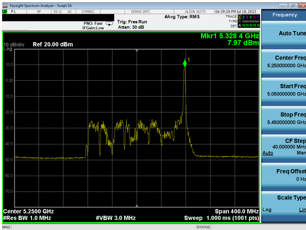
Plot 7-112. Power Spectral Density Plot MIMO ANT2 (160MHz BW 802.11ax – 26 Tones (UNII Band 1/2A) – Ch. 50)
