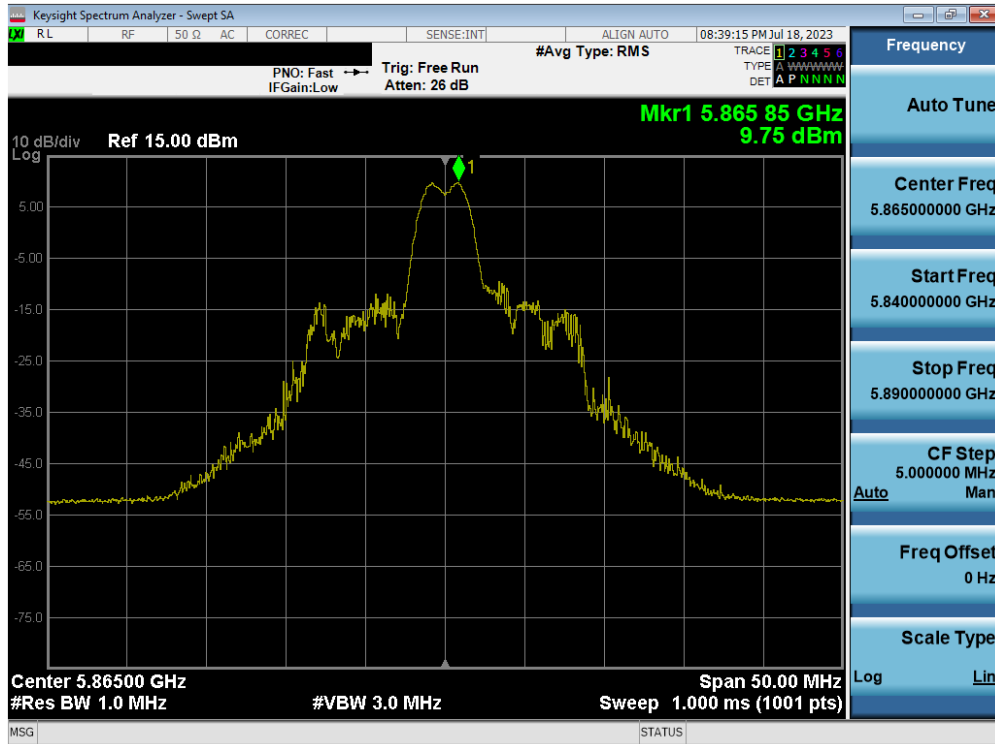
Plot 7-87. Power Spectral Density Plot MIMO ANT1 (20MHz BW 802.11ax – 26 Tones (UNII Band 4) – Ch. 173)
