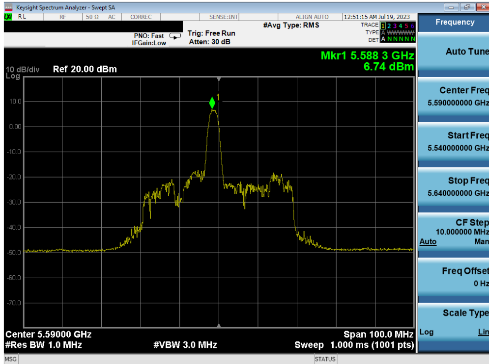
Plot 7-81. Power Spectral Density Plot MIMO ANT1 (40MHz BW 802.11ax – 26 Tones (UNII Band 2C) – Ch. 118)
