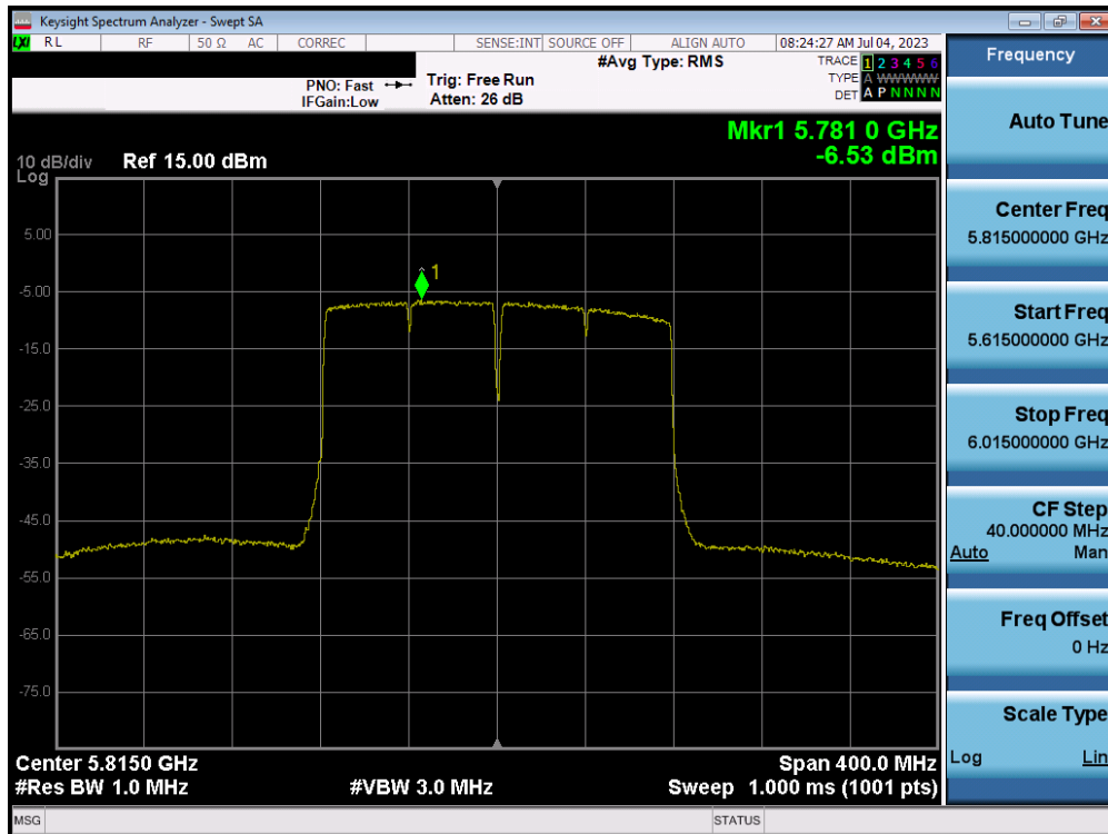
Plot 7-122. Power Spectral Density Plot MIMO ANT1 (160MHz BW 802.11ac (UNII Band 3/4) – Ch. 163)
