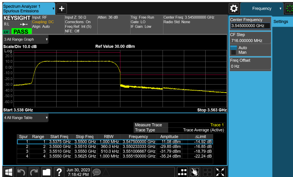
Plot 7-94. Upper ACP Plot (NR Band n77 (DoD) - 10MHz CP-OFDM-QPSK – Full RB – Ant F)
