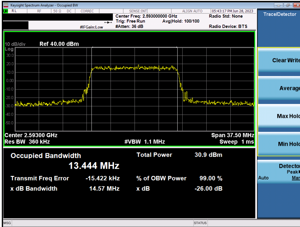
Plot 7-3. Occupied Bandwidth Plot (LTE Band 41(PC2) - 15MHz QPSK - Full RB - Ant1)
