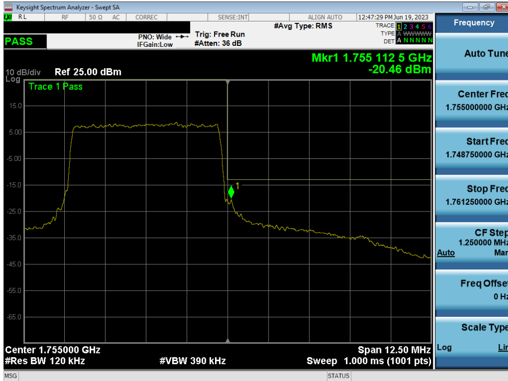
Plot 7-107. Upper Band Edge Plot (LTE Band 4 - 5MHz QPSK – Full RB - Ant1)
