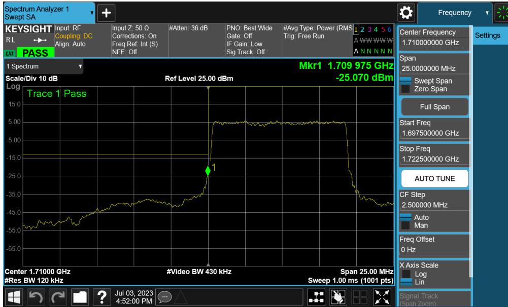
Plot 7-121. Lower Band Edge Plot (NR Band n66 – 10.0MHz - Full RB - Ant2)
