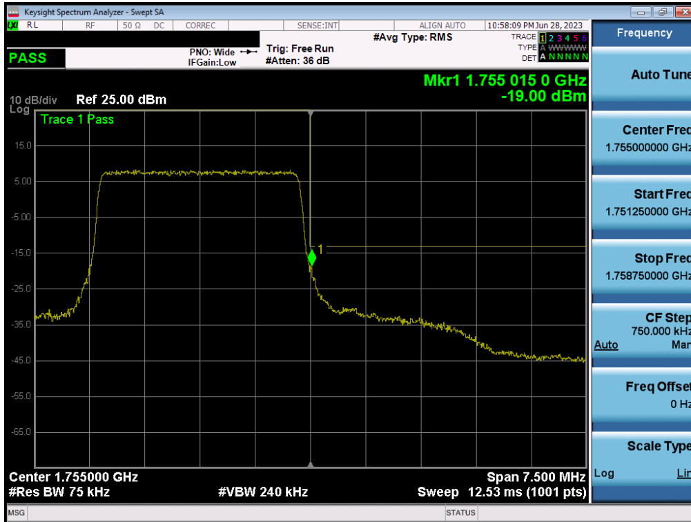
Plot 7-117. Upper Band Edge Plot (LTE Band 4 - 3MHz QPSK – Full RB - Ant2)
