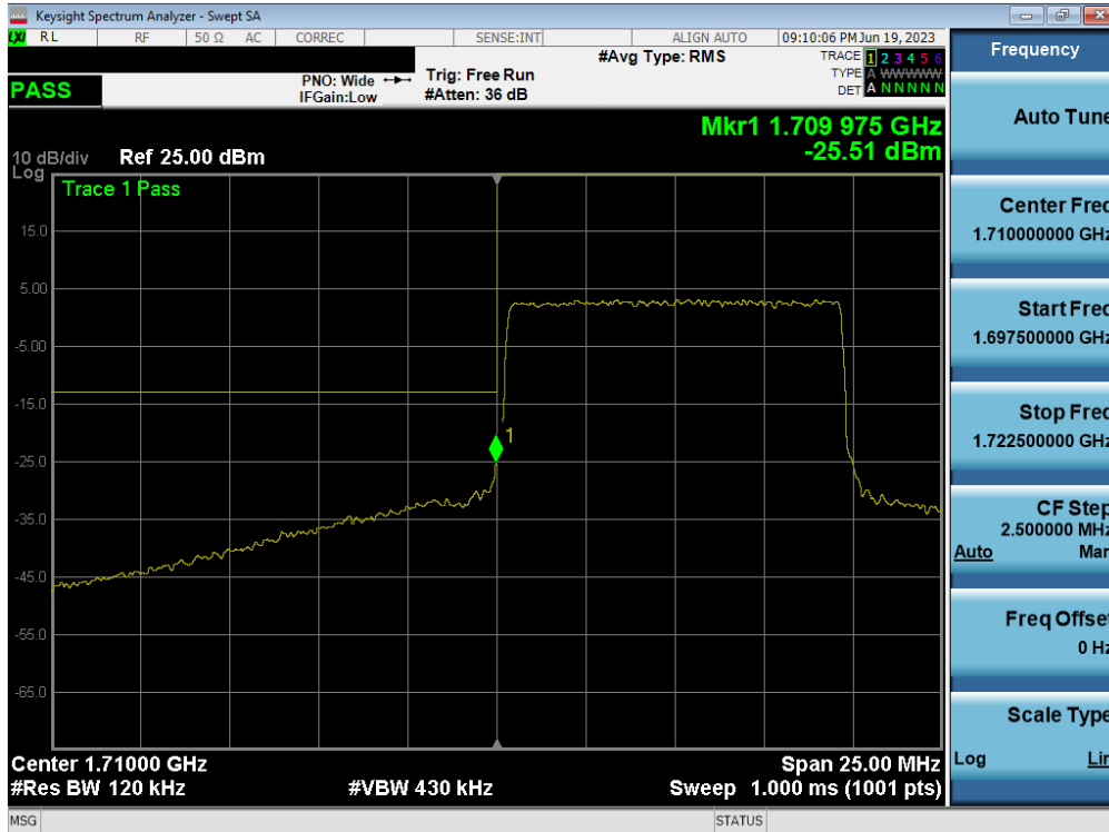
Plot 7-111. Lower Band Edge Plot (NR Band n66 - 10.0MHz - Full RB - Ant1)
