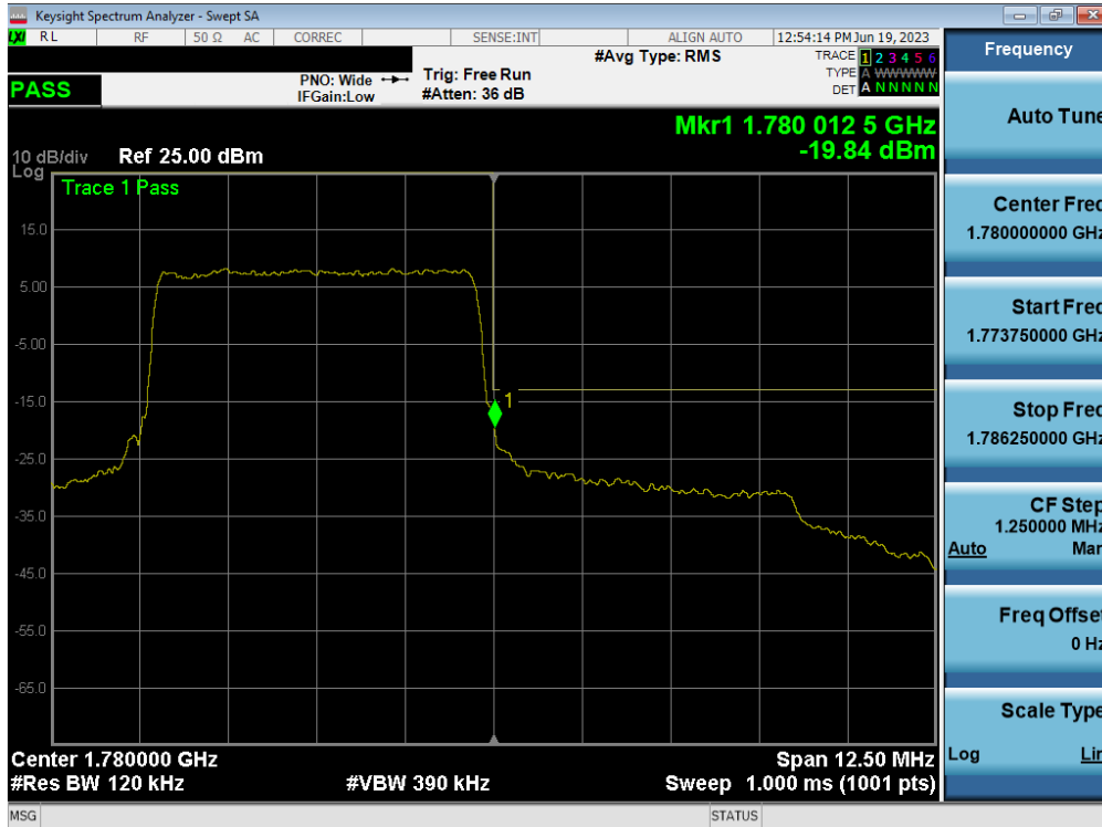
Plot 7-109. Upper Band Edge Plot (LTE Band 66 - 5MHz QPSK – Full RB - Ant1)
