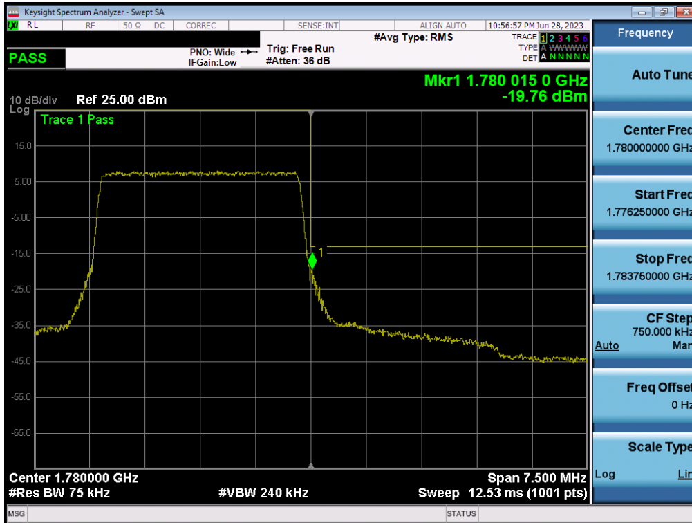
Plot 7-119. Upper Band Edge Plot (LTE Band 66 - 3MHz QPSK – Full RB - Ant2)
