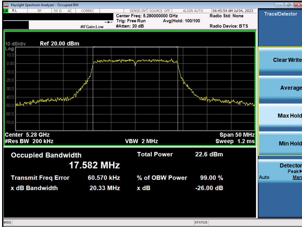
Plot 7-11. 26dB Bandwidth Plot MIMO ANT1 (20MHz BW 802.11n (UNII Band 2A) – Ch. 56)
