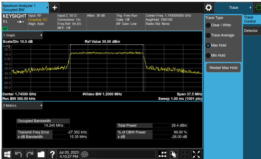
Plot 7-66. Occupied Bandwidth Plot (NR Band n66 - 15.0MHz CP-OFDM 16QAM - Full RB – Ant2)
