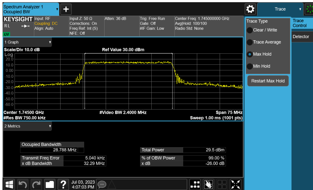
Plot 7-60. Occupied Bandwidth Plot (NR Band n66 - 30.0MHz CP-OFDM 16QAM - Full RB – Ant2)
