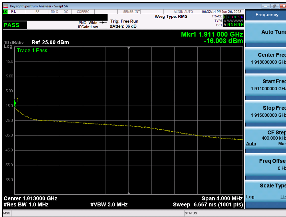
Plot 7-49. Extended Upper Band Edge Plot (WCDMA PCS – Ch. 9538 - Ant1)
