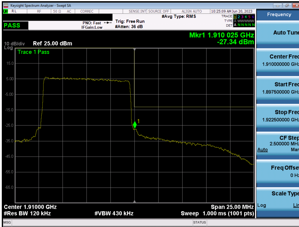
Plot 7-42. Upper Band Edge Plot (LTE Band 2 - 10MHz QPSK – Full RB - Ant1)
