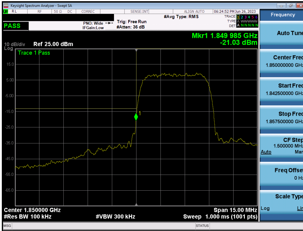
Plot 7-46. Lower Band Edge Plot (WCDMA PCS – Ch. 9262 - Ant1)
