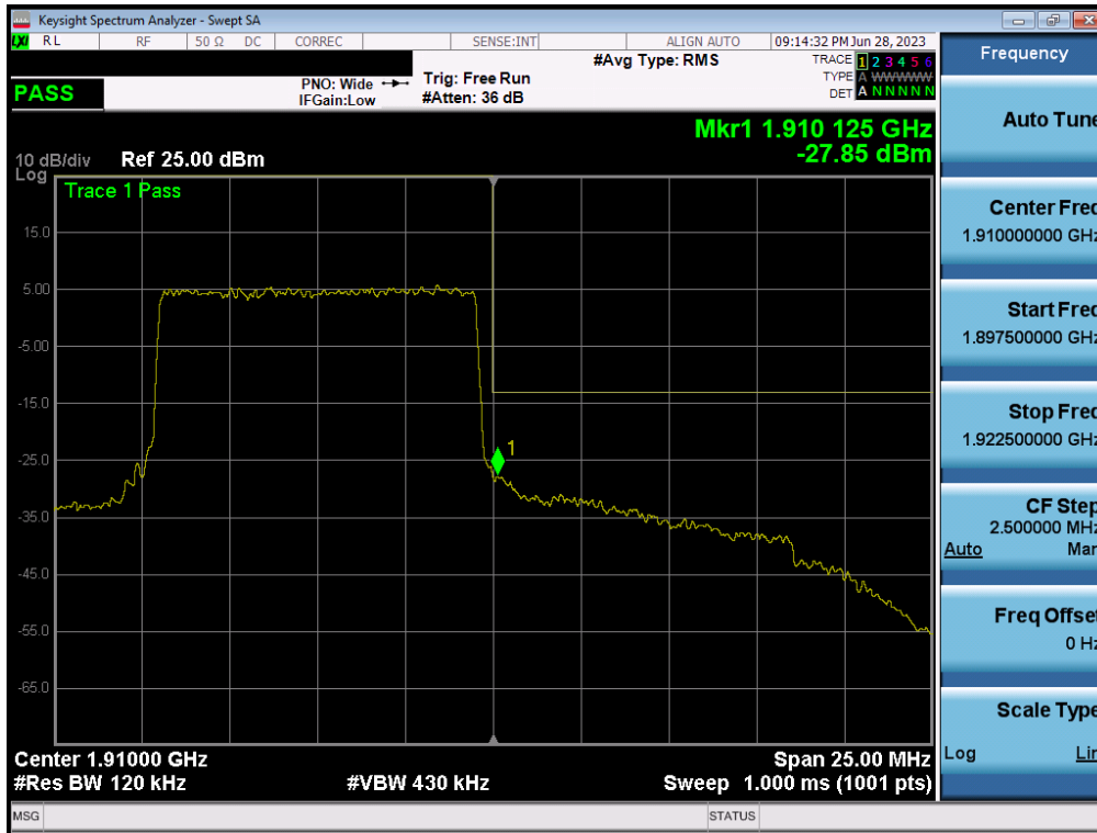
Plot 7-52. Upper Band Edge Plot (LTE Band 2 - 10MHz QPSK – Full RB - Ant2)
