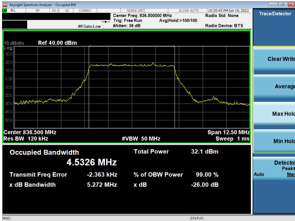
Plot 7-20. Occupied Bandwidth Plot (NR Band n5 - 5MHz \pi/2 BPSK - Full RB)
