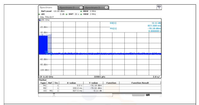
Channel move time =  $0.827 \frac{500 \text{ s}}{1000}$ Closing time =  $0.000 \frac{625 \text{ s}}{1000}$  x 82 =  $0.051 \frac{250 \text{ s}}{1000}$
