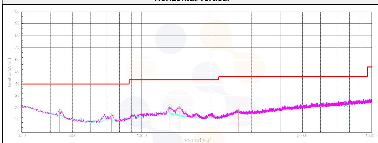
**Test results (Above 1 000 MHz)****802.11b\_2 412 MHz**
