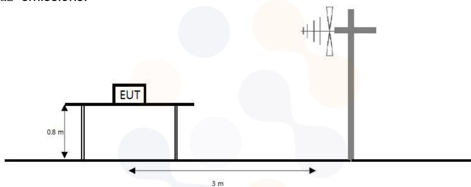
The diagram below shows the test setup that is utilized to make the measurements for emission from 1 GHz to the tenth harmonic of the highest fundamental frequency or to 40 GHz emissions, whichever is lower.
