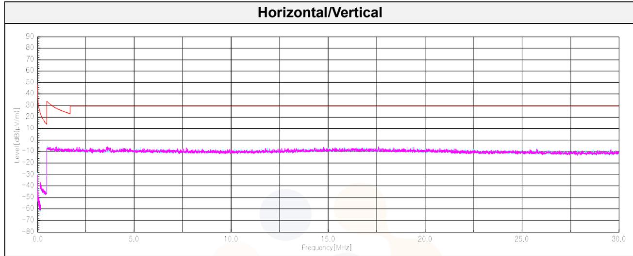
**Test results (Below 1 000 MHz) –Worst case: 2 Mbits/s(37 Bytes) 2 440 MHz**
