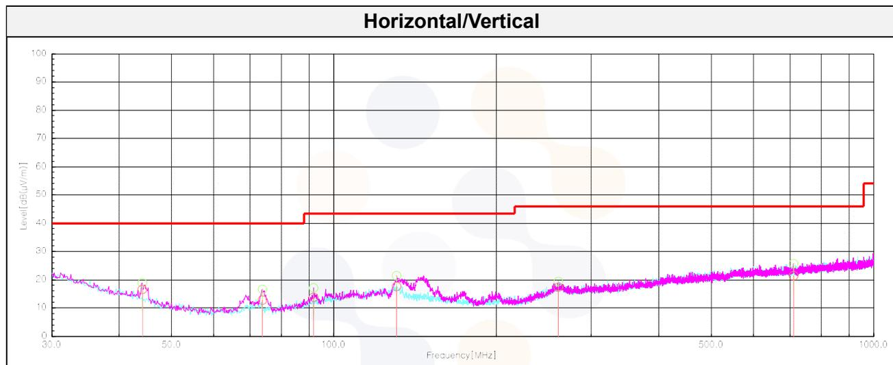
**Test results (Above 1 000 MHz)\_1 Mbits/s(37 Bytes)**
