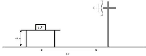
The diagram below shows the test setup that is utilized to make the measurements for emission from 1 to the tenth harmonic of the highest fundamental frequency or to 40 to emissions, whichever is lower.
