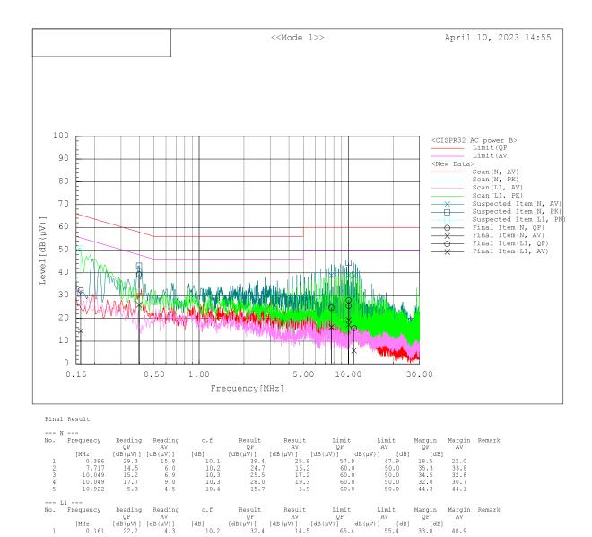
Note 1) Two graphs measured for both Live(L1) and Neutral(N) of the LISN are combined into one graph Note 2) Level (QP and/or CAV) = Meter Reading (QP and/or CAV) + Corr. (LISN Insertion Loss + Cable Loss) Margin (QP and/or CAV) = Limit – Level (QP and/or CAV)
