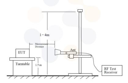
The diagram below shows the test setup for substituted method.
