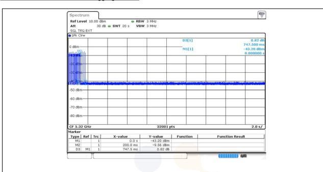
Channel move time = 0.747 500 sClosing time =  $0.000 625 \text{ s} \times 21 = 0.013 125 \text{ s}$
