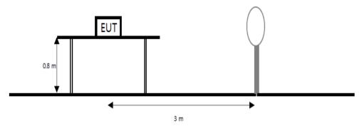
The diagram below shows the test setup that is utilized to make the measurements for emission from 30 Mz to 1 Gz emissions.
