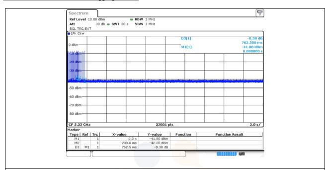
Channel move time =  $0.762 \, 500 \, \text{s}$ Closing time =  $0.000 \, 625 \, \text{s} \, \text{x} \, 8 = 0.005 \, 000 \, \text{s}$
