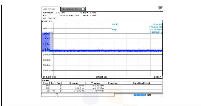
(Closing time: Burst unit time(20 s / 32 001 points) \* Number of burst(between 2 markers))
