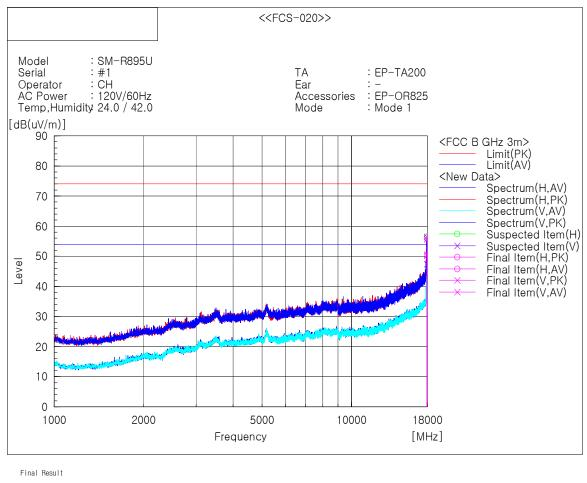
Limit PK [dB(uV/m)] 74.0 74.0 74.0 Limit AV [dB(uV/m)] 54.0 54.0 54.0 Margin PK [dB] 17.9 17.6 Margin AV [dB] 3.6 3.8 3.4 No. Frequency (P) Reading Reading c.f Result Result Height Angle Remark C.1 Hesult PK [dB(1/m)] [dB(uV/m)] 34.2 56.1 34.3 56.4 34.4 56.4 AV [dB(uV/m)] 50.4 50.2 50.6 PK [dB(uV)] 21.9 22.1 22.0 (dB(uV)) 16.2 15.9 16.2
