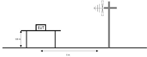
The diagram below shows the test setup that is utilized to make the measurements for emission from 1  $\oplus$  to the tenth harmonic of the highest fundamental frequency or to 40  $\oplus$  emissions, whichever is lower.
