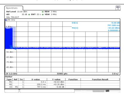
Channel move time = 0.797500 sClosing time =  $0.000625 \text{ s} \times 36 = 0.022500 \text{ s}$
