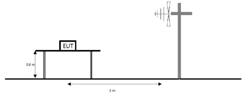
The diagram below shows the test setup that is utilized to make the measurements for emission from 1  $\mbox{d}$  to the tenth harmonic of the highest fundamental frequency or to 40  $\mbox{d}$  emissions, whichever is lower.
