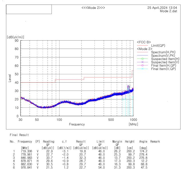
Note1) Receiving antenna polarization : Horizontal, Vertical Test Distance : 3 m, Antenna Height : 1 to 4 meters Result (QP) = Reading (QP) + c.f (Antenna Factor + Cable Loss - Amp. Gain) Margin (QP) = Limit – Level (QP) QP = Quasi-Peak, c.f = Correction Factor
