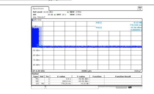
Channel move time = 0.776 250 sClosing time =  $0.000 625 \text{ s} \times 12 = 0.007 500 \text{ s}$
