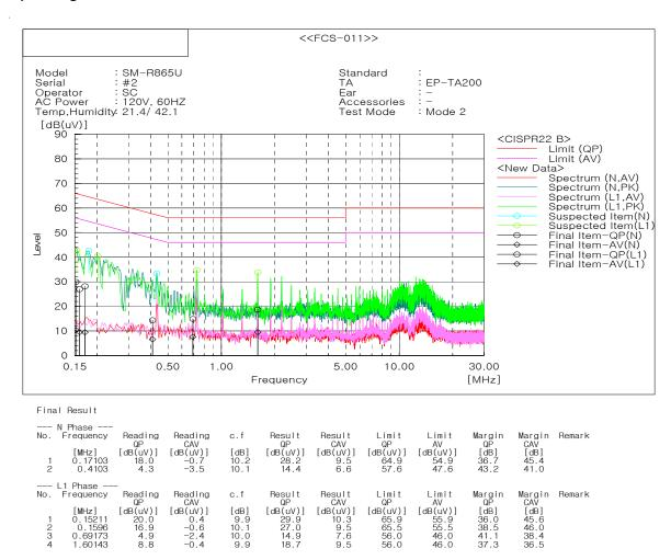
Note 1) Two graphs measured for both Live(L1) and Neutral(N) of the LISN are combined into one graph Note 2) Level (QP and/or CAV) = Meter Reading (QP and/or CAV) + Corr. (LISN Insertion Loss + Cable Loss) Margin (QP and/or CAV) = Limit – Level (QP and/or CAV) QP = Quasi-Peak, CAV = CISPR-Average, Corr. = Correction Factor.
