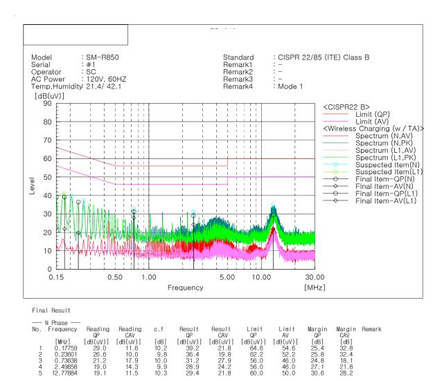
Note 1) Two graphs measured for both Live(L1) and Neutral(N) of the LISN are combined into one graph Note 2) Level (QP and/or CAV) = Meter Reading (QP and/or CAV) + Corr. (LISN Insertion Loss + Cable Loss) Margin (QP and/or CAV) = Limit – Level (QP and/or CAV) QP = Quasi-Peak, CAV = CISPR-Average, Corr. = Correction Factor.
