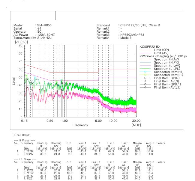
Note 1) Two graphs measured for both Live(L1) and Neutral(N) of the LISN are combined into one graph Note 2) Level (QP and/or CAV) = Meter Reading (QP and/or CAV) + Corr. (LISN Insertion Loss + Cable Loss) Margin (QP and/or CAV) = Limit – Level (QP and/or CAV)
