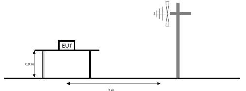
The diagram below shows the test setup that is utilized to make the measurements for emission from 1 GHz to the tenth harmonic of the highest fundamental frequency or to 40 GHz emissions, whichever is lower.
