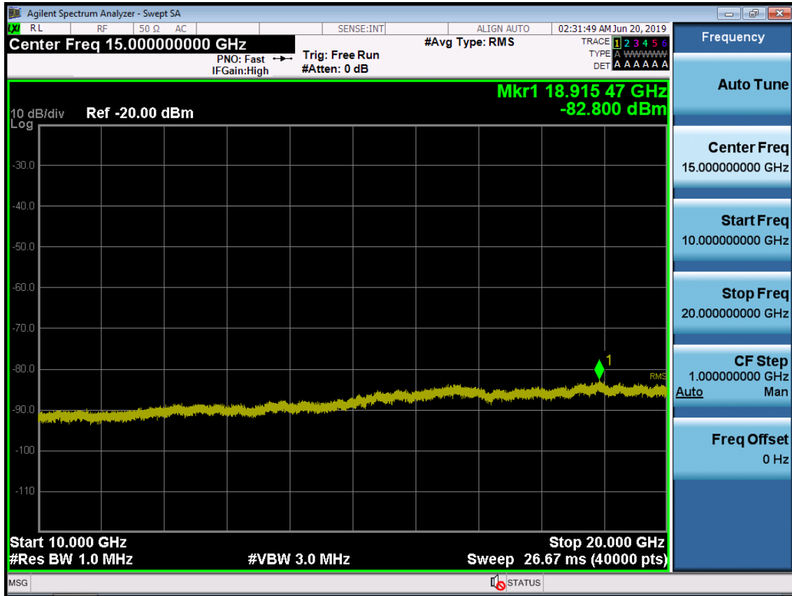
BAND 66. Conducted Spurious Plot_2 (131997ch_5MHz_QPSK_RB 1_0)
