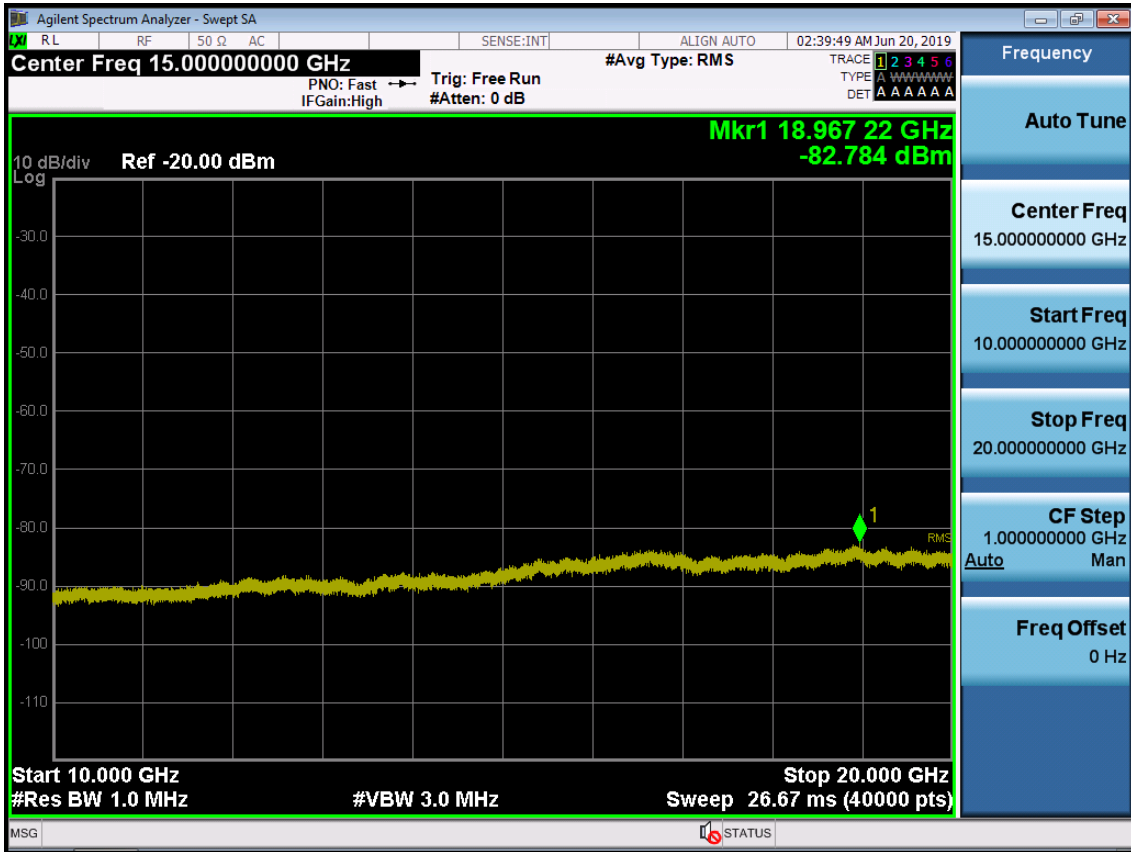
BAND 66. Conducted Spurious Plot_2 (132322ch_10MHz_QPSK_RB 1_0)
