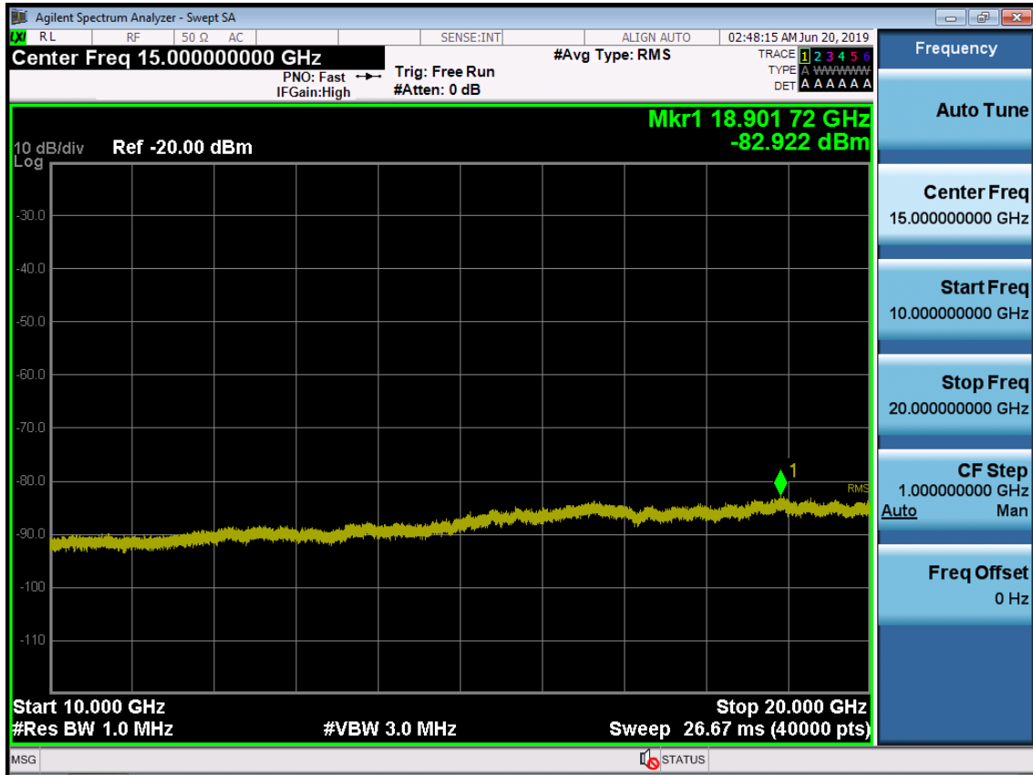
BAND 66. Conducted Spurious Plot_2 (132597ch_15MHz_QPSK_RB 1_0)
