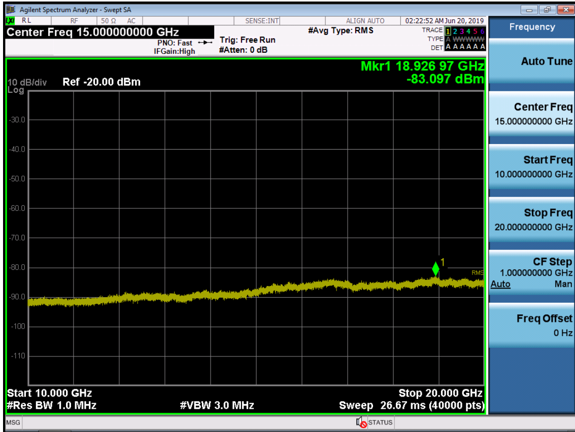
BAND 66. Conducted Spurious Plot_2 (132665ch_1.4MHz_QPSK_RB 1_0)
