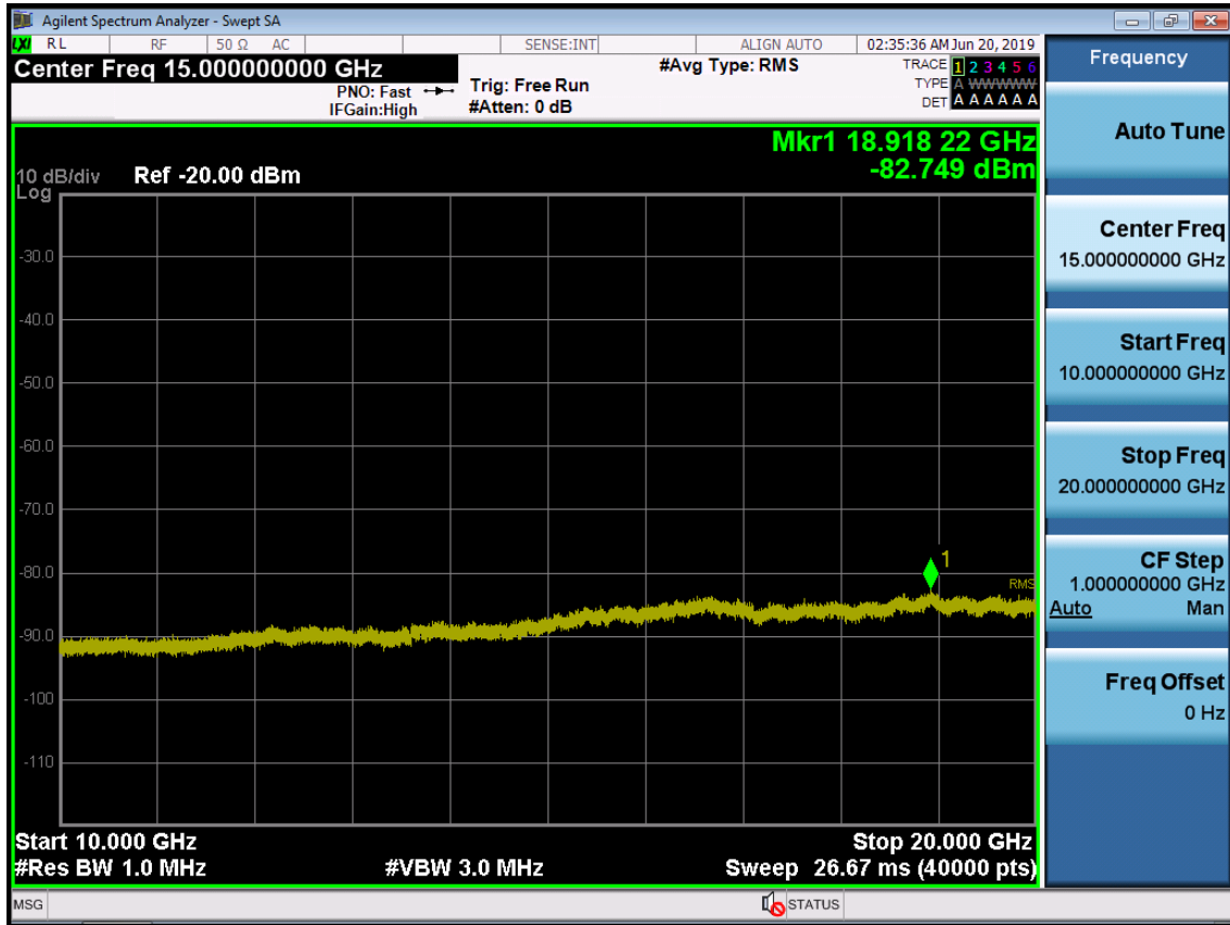
BAND 66. Conducted Spurious Plot_2 (132647ch_5MHz_QPSK_RB 1_0)
