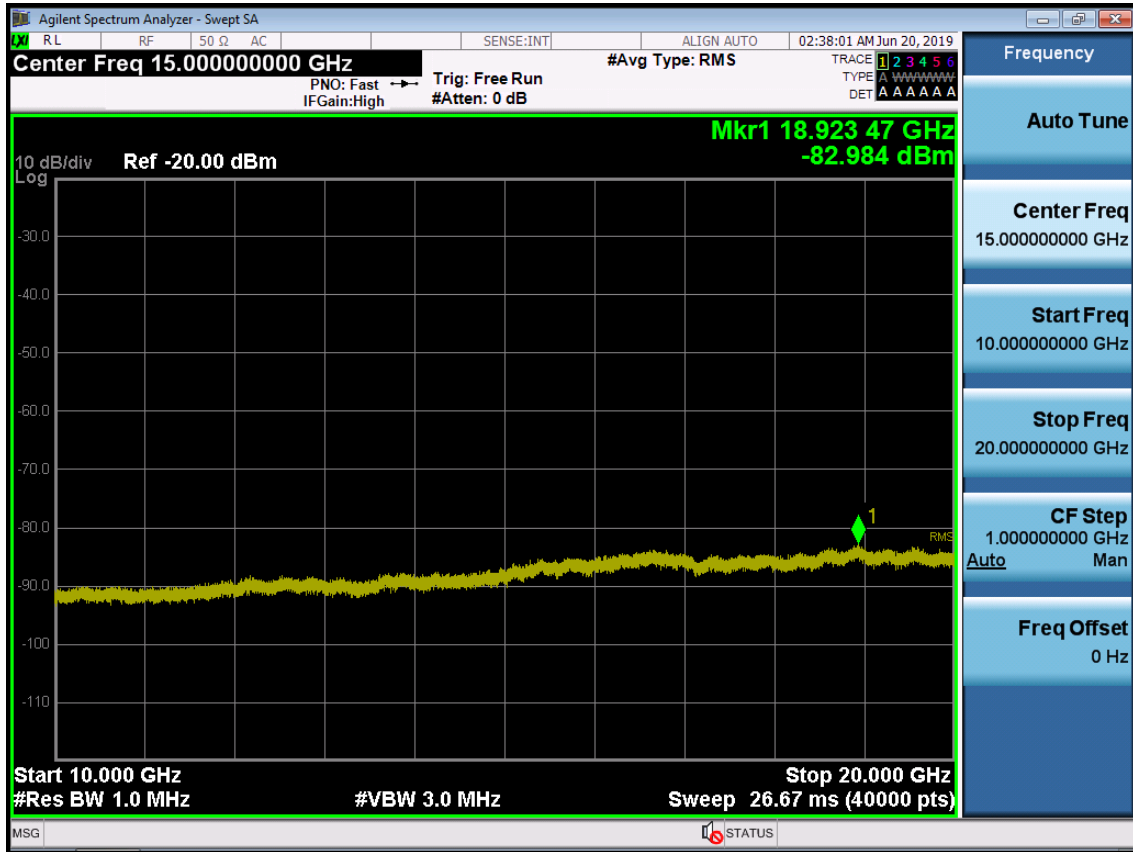
BAND 66. Conducted Spurious Plot_2 (132022ch_10MHz_QPSK_RB 1_0)
