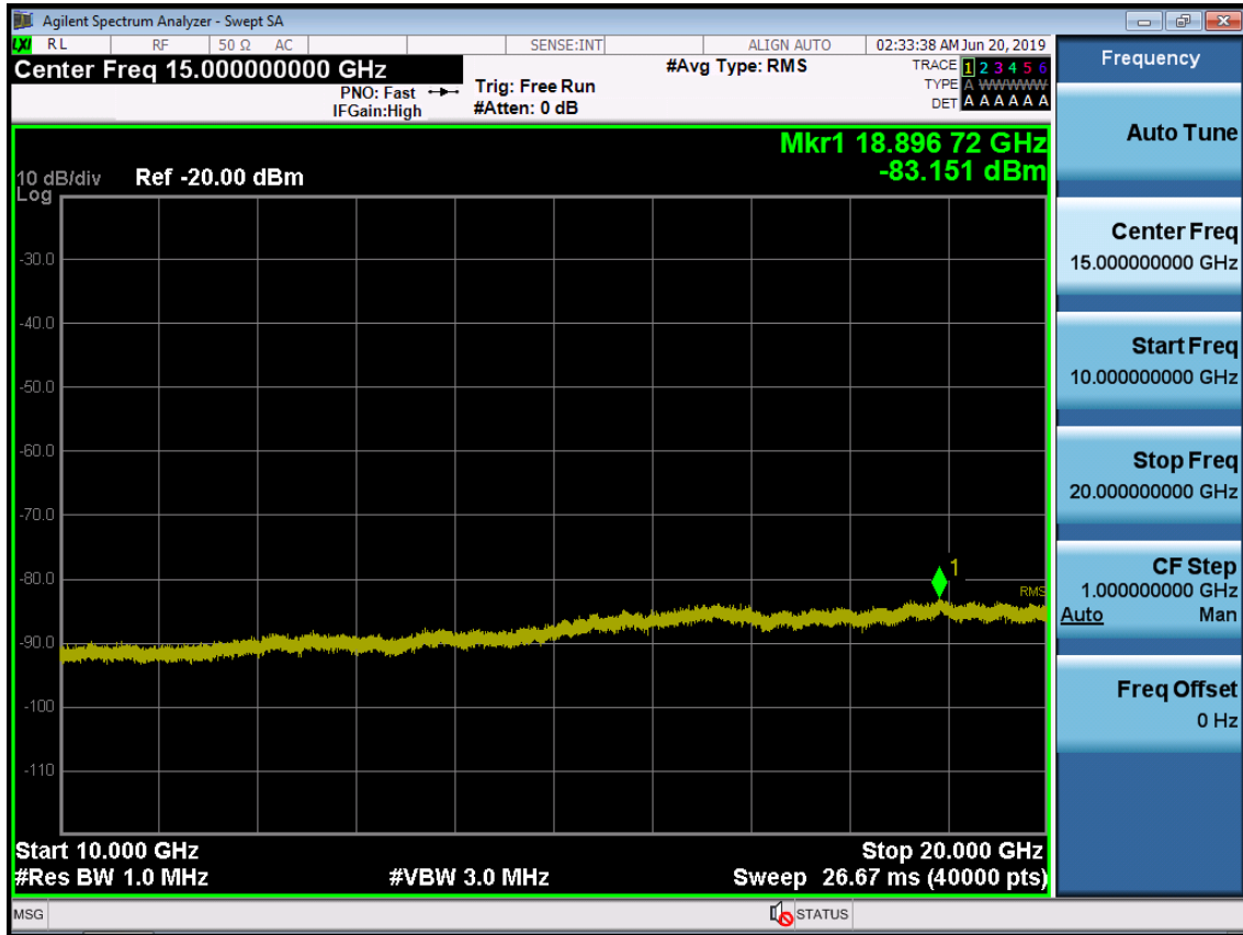
BAND 66. Conducted Spurious Plot_2 (132322ch_5MHz_QPSK_RB 1_0)
