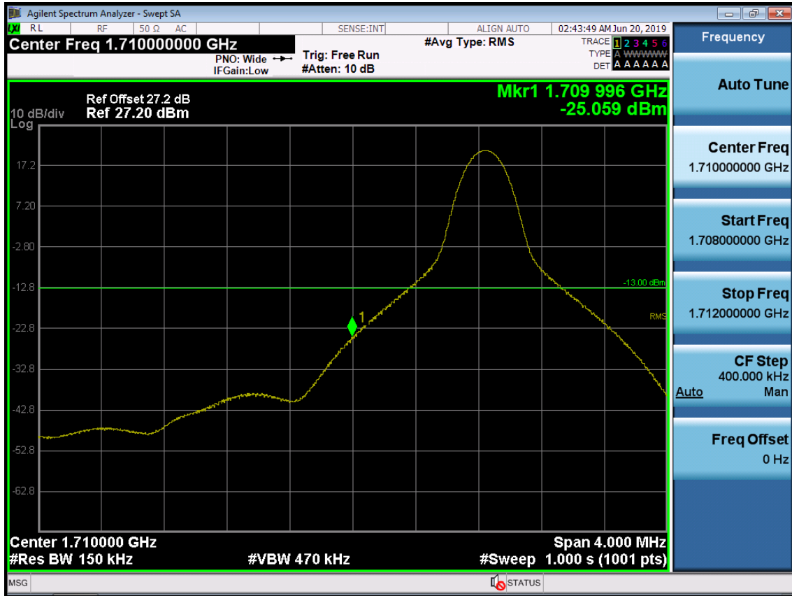
BAND 66. Lower Band Edge Plot (15M BW Ch.132047 QPSK RB 1, Offset 0) -1
