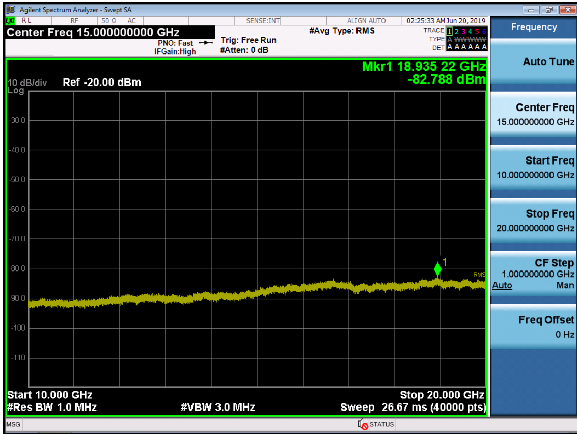
BAND 66. Conducted Spurious Plot_2 (131987ch_3MHz_QPSK_RB 1_0)
