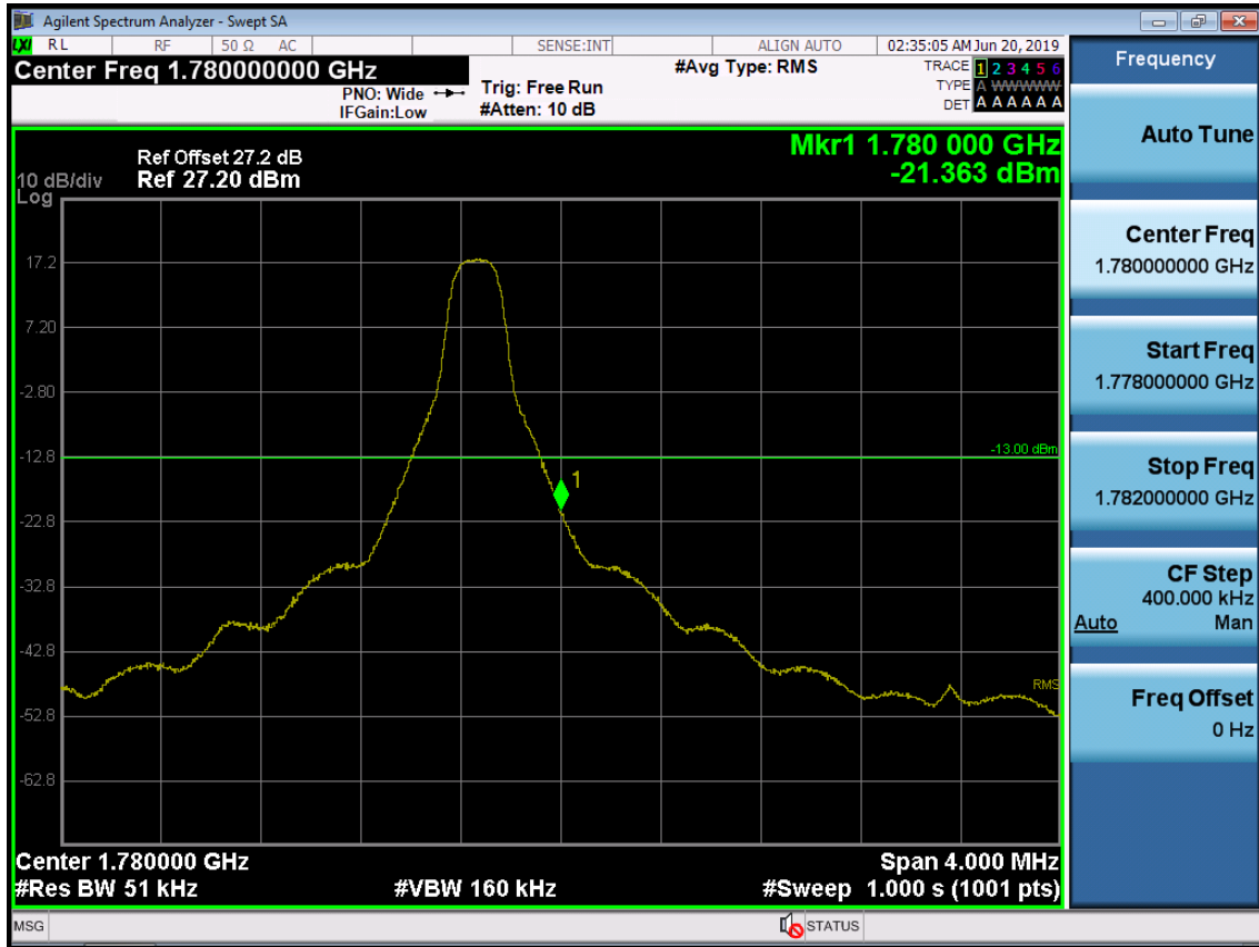
BAND 66. Upper Band Edge Plot (5M BW Ch.132647 QPSK_RB1_Offset 24) -1
