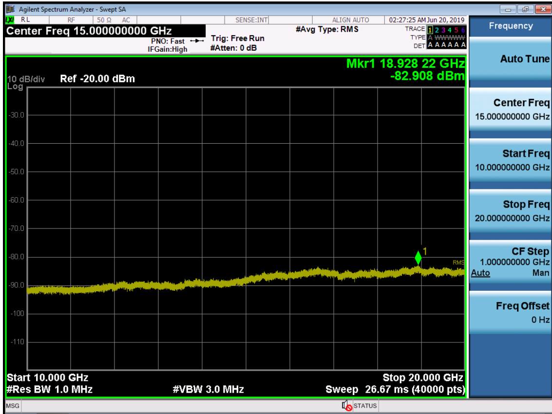
BAND 66. Conducted Spurious Plot_2 (132322ch_3MHz_QPSK_RB 1_0)
