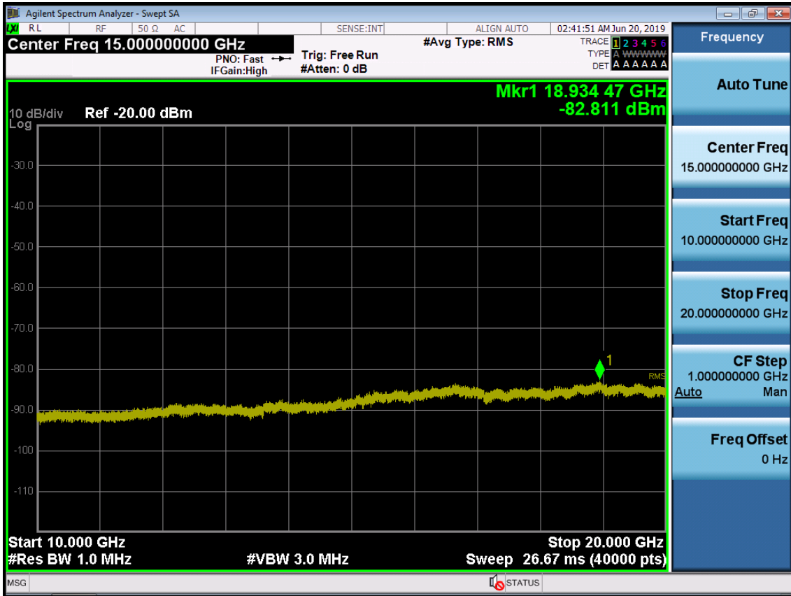
BAND 66. Conducted Spurious Plot_2 (132622ch_10MHz_QPSK_RB 1_0)
