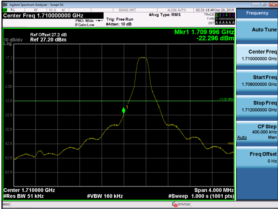
BAND 66. Lower Band Edge Plot (5M BW Ch.131997 QPSK RB 1, Offset 0) -1
