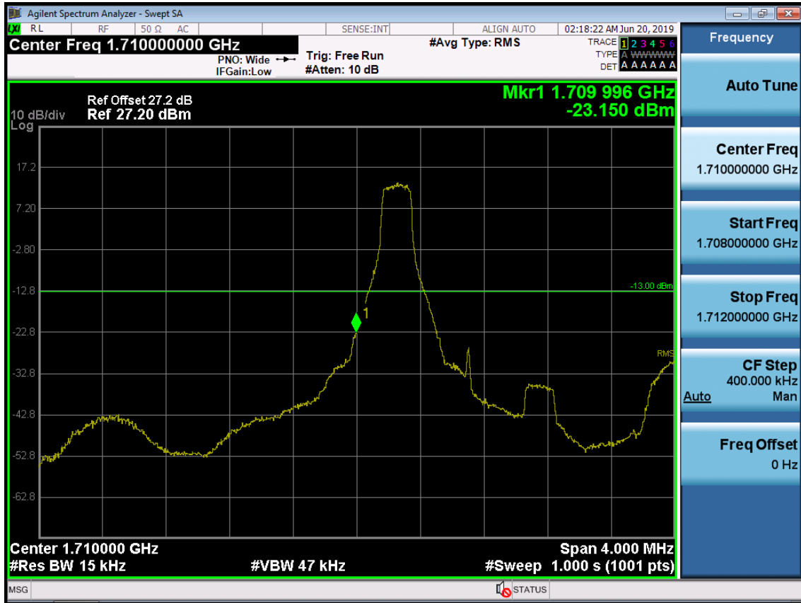
BAND 66. Lower Band Edge Plot (1.4M BW Ch.131979 QPSK RB 1, Offset 0) -1
