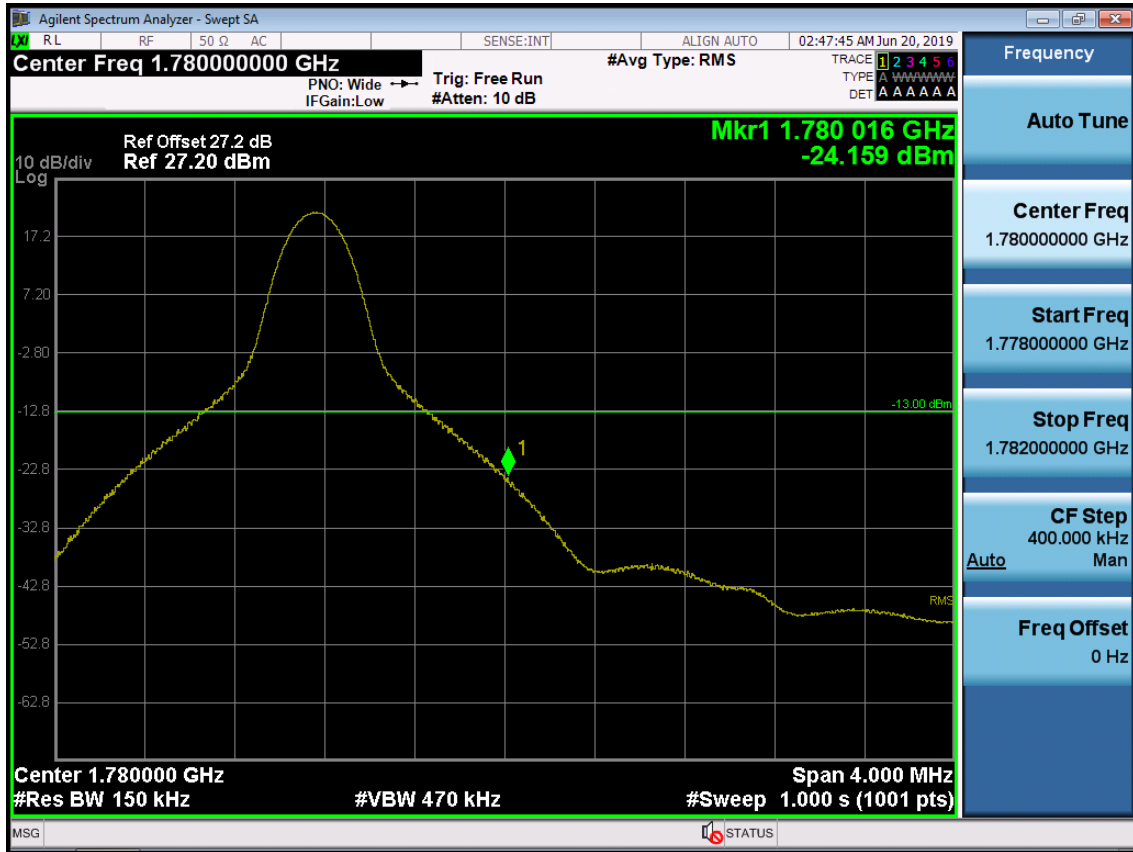
BAND 66. Upper Band Edge Plot (15M BW Ch.132597 QPSK_RB1_Offset 74) -1
