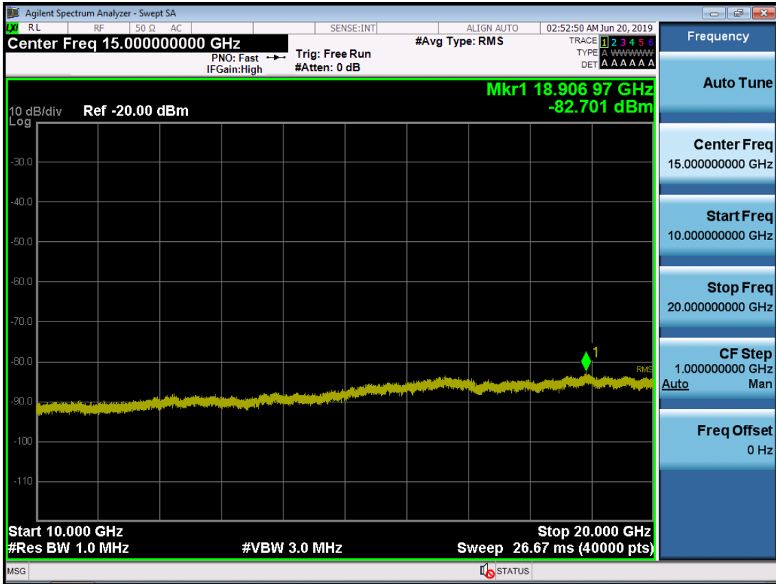
BAND 66. Conducted Spurious Plot_2 (132322ch_20MHz_QPSK_RB 1_0)
