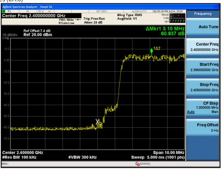
Test Plots with hopping (8DPSK)
