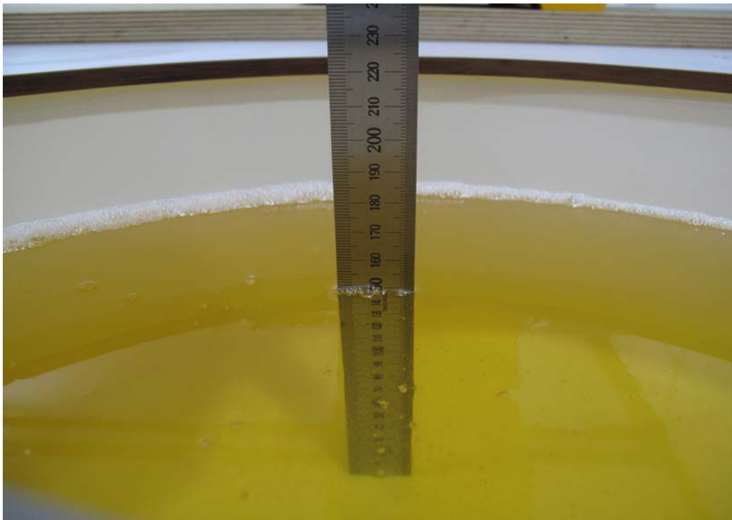
2 GHz (Head) Tissue Simulating Liquid, Depth: 150 mm
